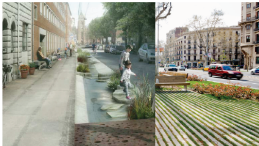
Small-scale channel (1m) + permeable pavers with underground storage (hardstand areas at intersections)
