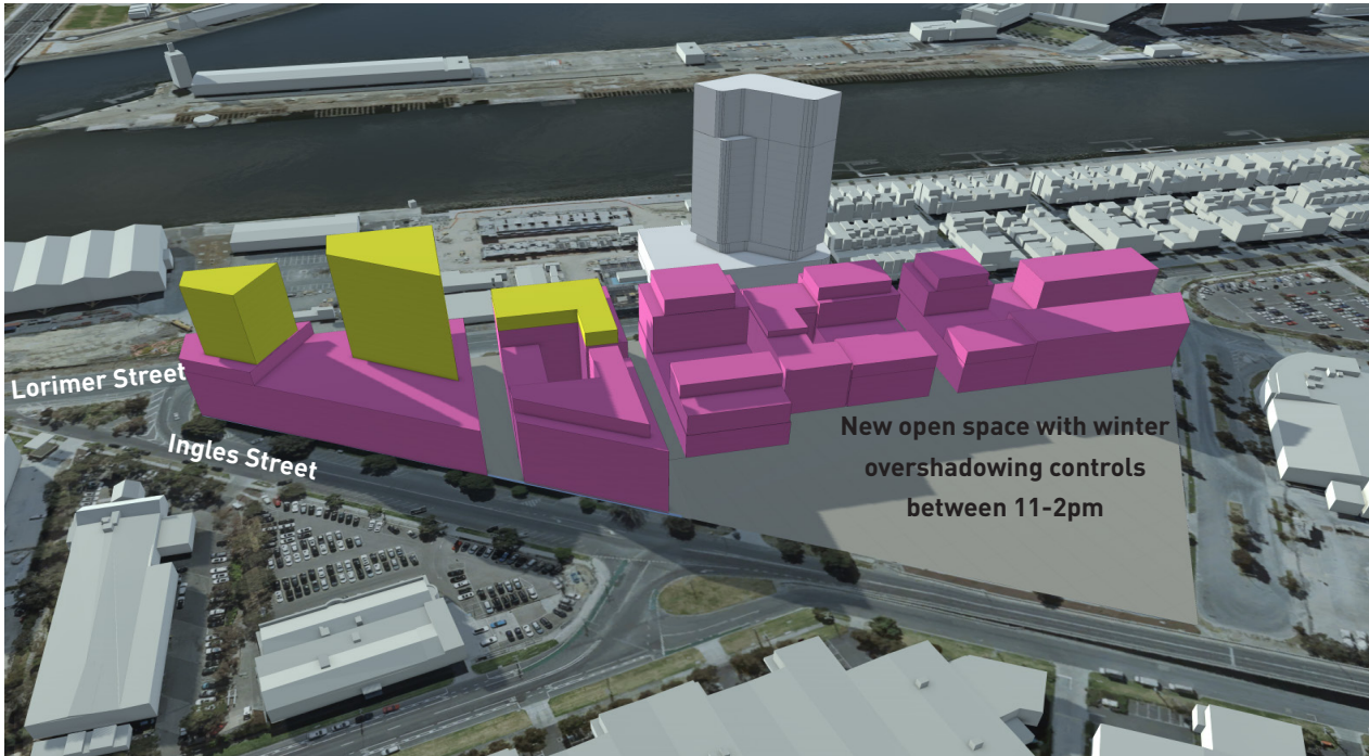
Figure 17 An alternative design outcome for the block bounded by Lorimer Street, Ingles Street and Rogers Street. In this example all sites are also modelled to the proposed FAR of 5.4 and in compliance with the built envelope controls (including overshadowing requirements for the new park). The site on the corner of Lorimer Street and Ingles Street incorporates additional yield delivered through a FAU (illustrated in yellow). This equates to 177 apartments of which 20 would be dedicated to affordable housing.
