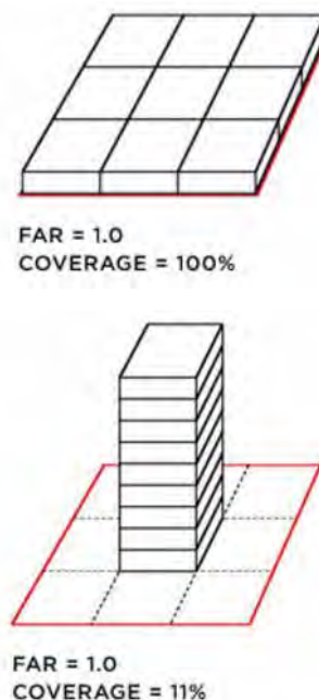
Figure 14: Example of a FAR of 1:1 delivering a 1 storey high building with high site coverage (100%) (above) and 9 storey building with low site coverage (11%) (below) - Source: Density Atlas
