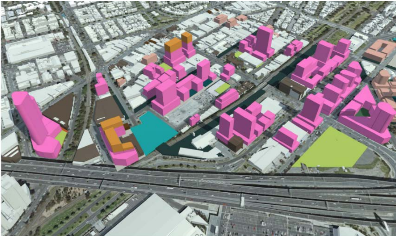
Figure 4 Montague perspective view (from north-east): In this illustration all sites are also modelled to the proposed FAR of 6.3 (core area) and 3.6 (non-core area) and in compliance with the built envelope controls (including overshadowing requirements). This demonstrates a variety of potential design responses that are possible within the proposed controls.
