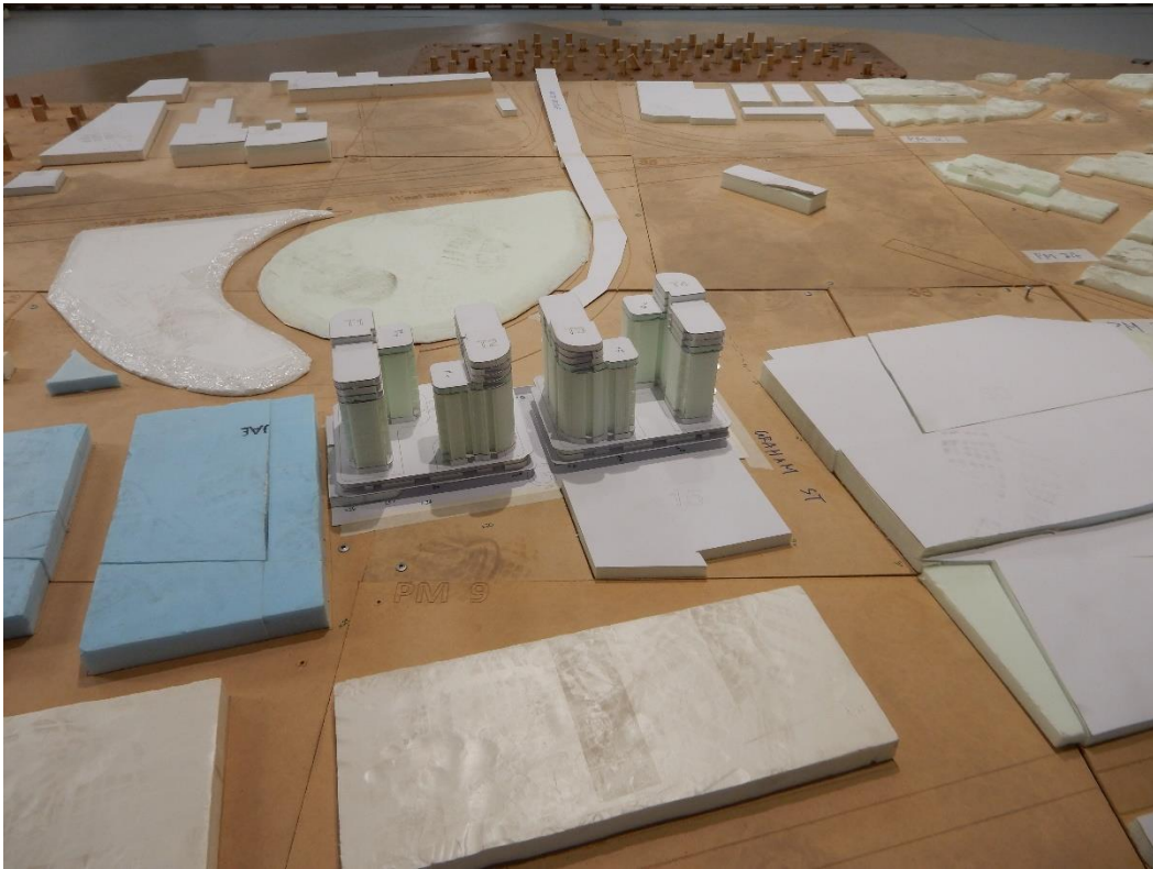
Figure 2 – View from the south of the 1/400 scale Proposed Configuration model of the 541 Graham Street Development in the wind tunnel
