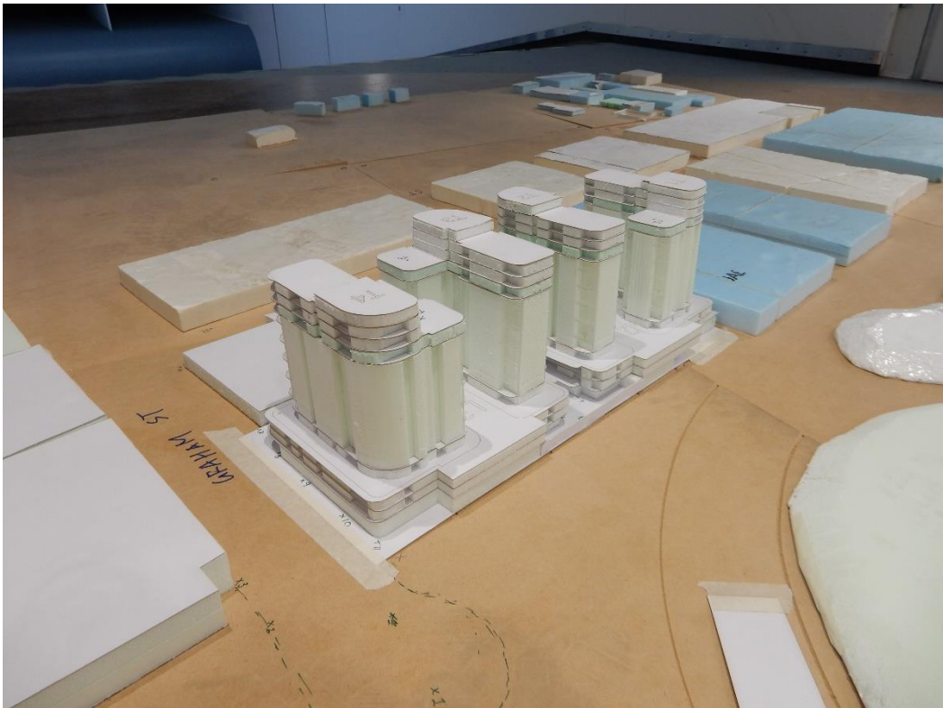
Figure 3 – Close-up view from the northeast of the 1/400 scale Proposed Configuration model of the 541 Graham Street Development in the wind tunnel.
