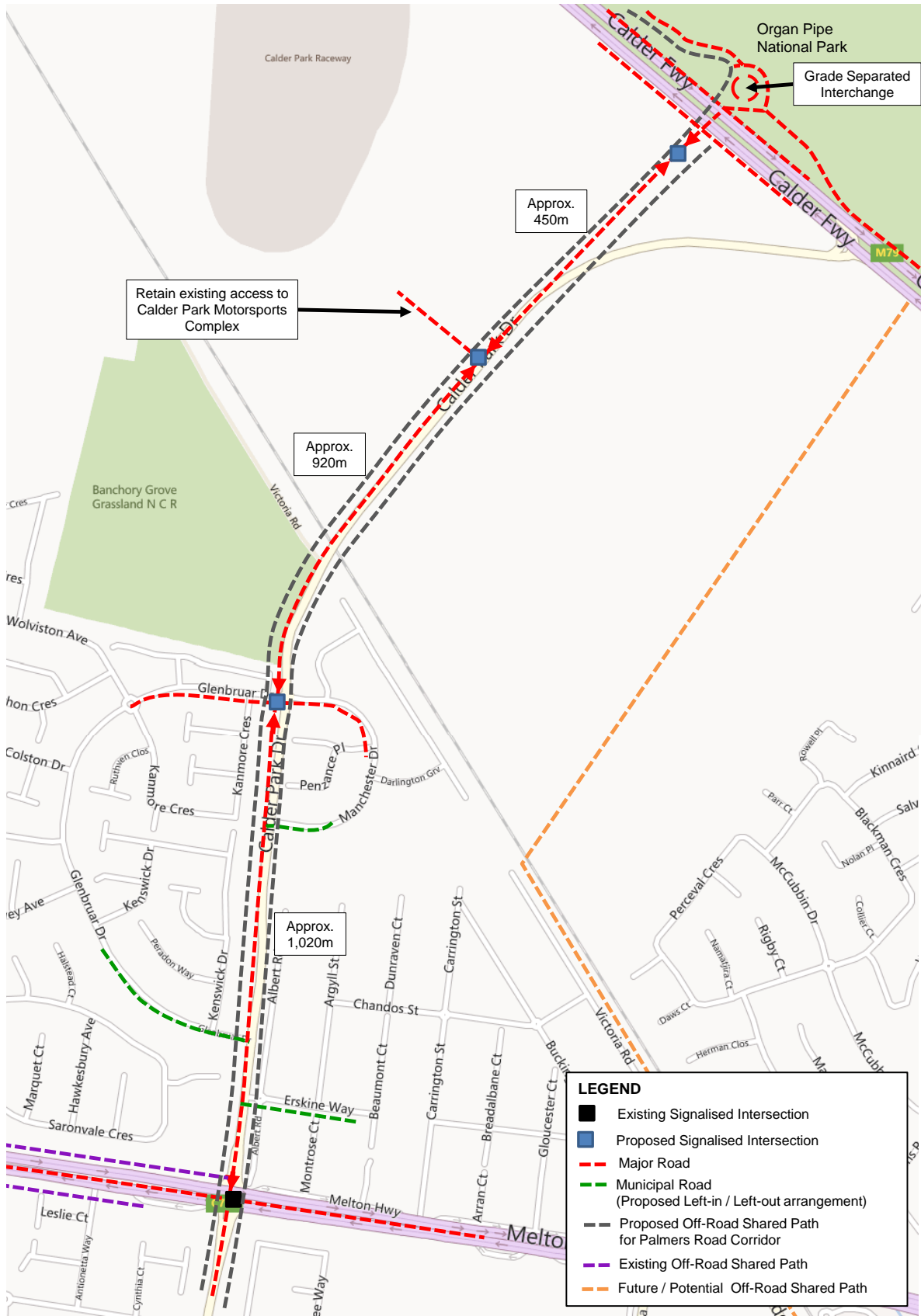
Figure 11 Proposed location and spacing of signalised intersections between Calder Park Drive and Melton Highway and Calder Freeway
