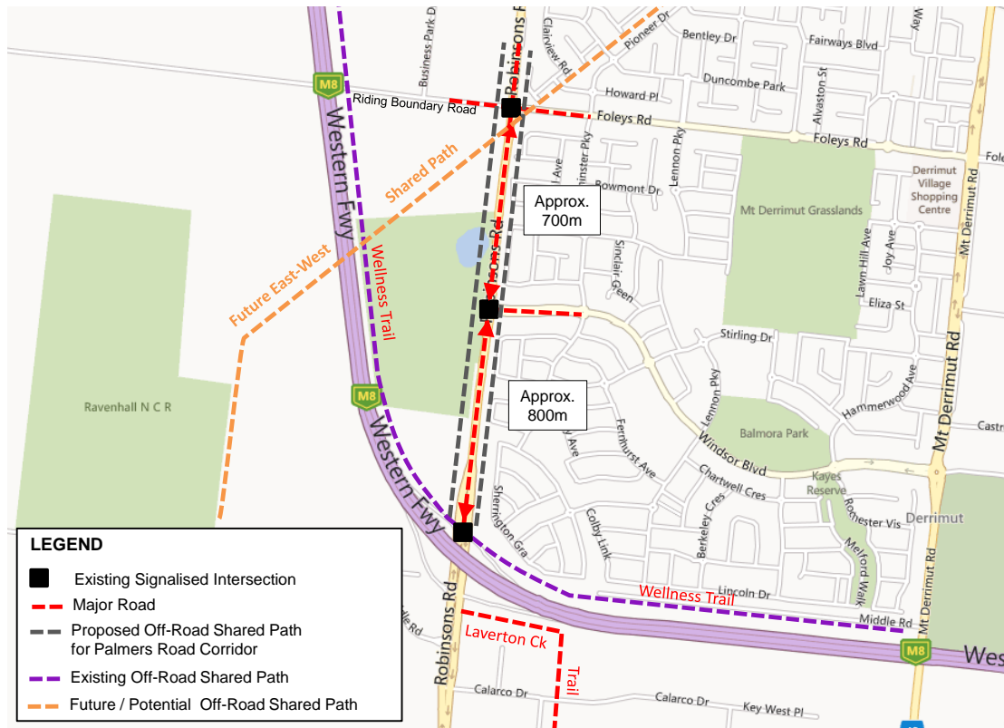
Figure 7 Proposed location and spacing of signalised intersections between Western Freeway and Riding Boundary Road / Foleys Road
