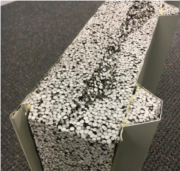
Figure 27. Example of EPS in phenolic resin matrix, Photo by CSIRO
