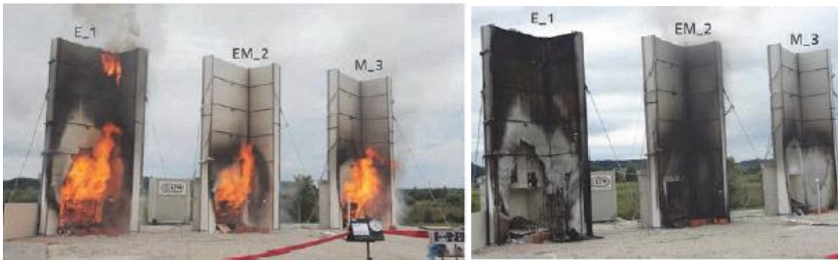
Figure 93. EIFS BS 8414 tests at 21 minutes and after suppression [169]
