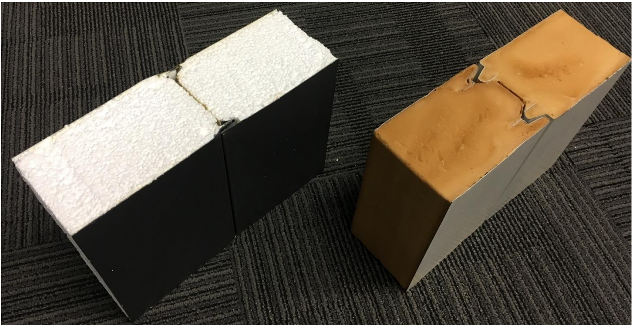
Figure 2. Typical ISP with interlocking slip joints, EPS core (left), PIR core (right). Photos by CSIRO
