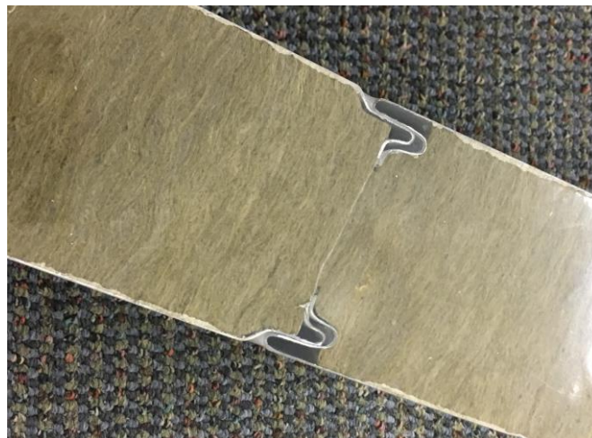
Figure 23. Example of Mineral Wool Core ISP. Photo by CSIRO
