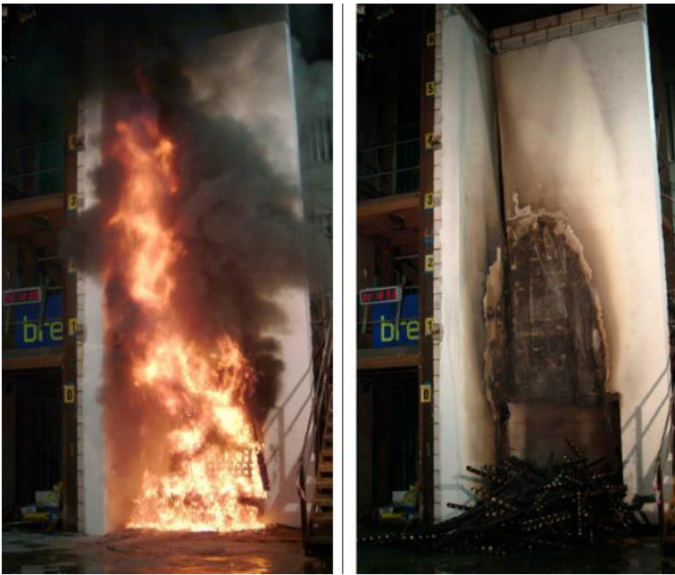
Figure 92. BRE BS 8414 test on 200 mm EPS with organic render resulting in BR 135 criteria fail before and after test suppression [159]
