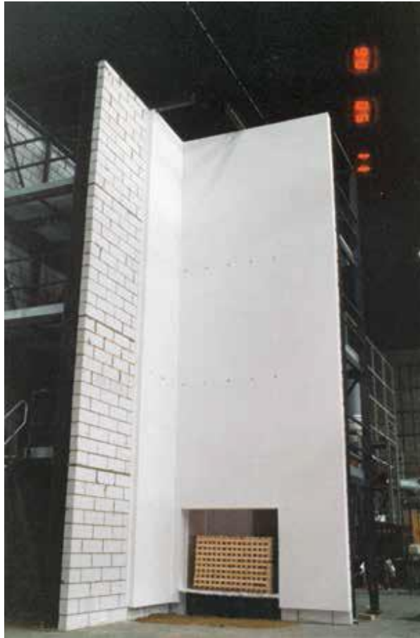
Figure 79. BS8414-1 test rig (from BRE report BR135 [157] )
