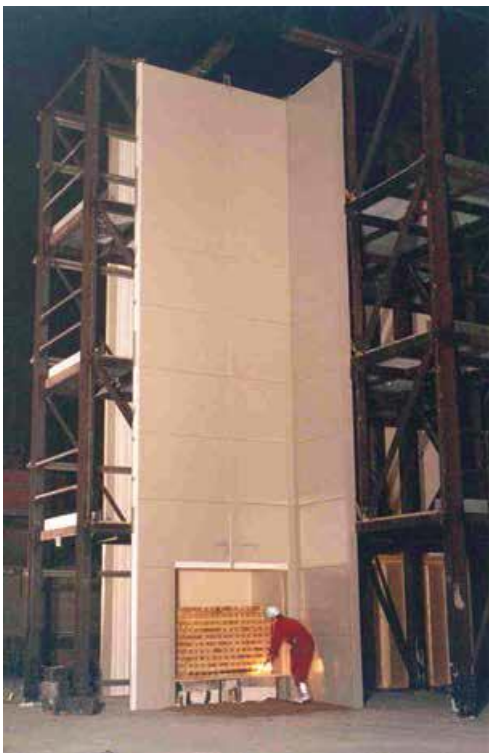
Figure 80. BS8414-2 test rig (from BRE report BR135 [157] )
