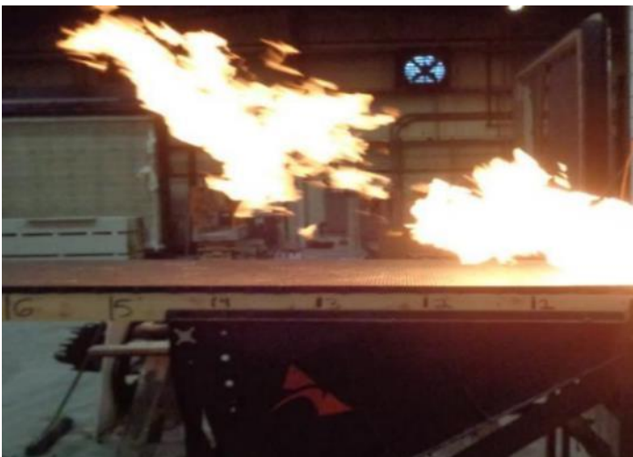
Figure 73. ASTM E-108 Spread of flame test
