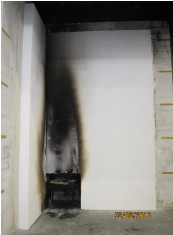
Figure 81. DIN 4102-20 (Draft) test rig (From BRE Global [159] )
