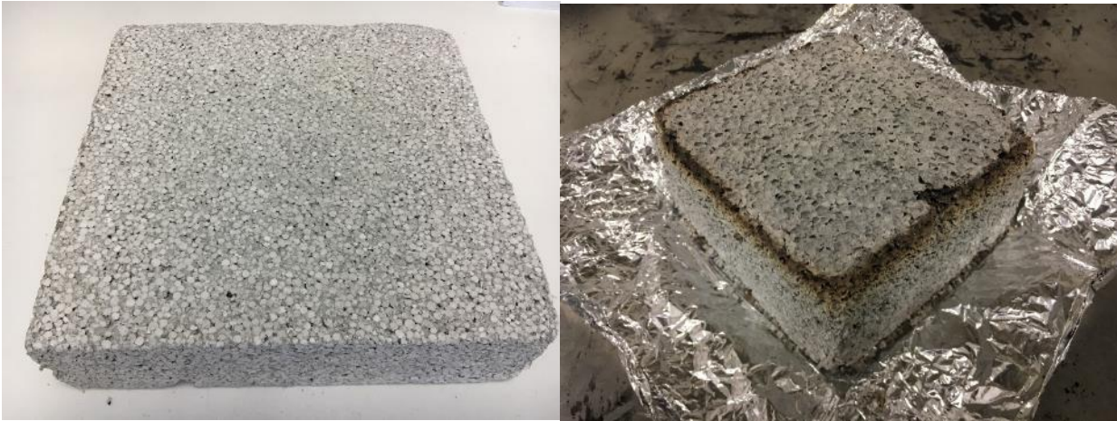
Figure 26. Compolcrete prior to cone calorimeter test (left) and after cone calorimeter test (right) – All photos by CSIRO
