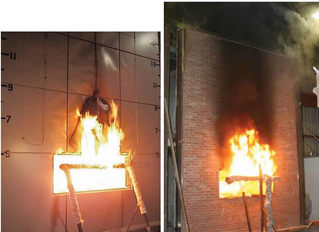
Figure 83. Front view of typical NFPA 285 test (from Hansbro [162] )
