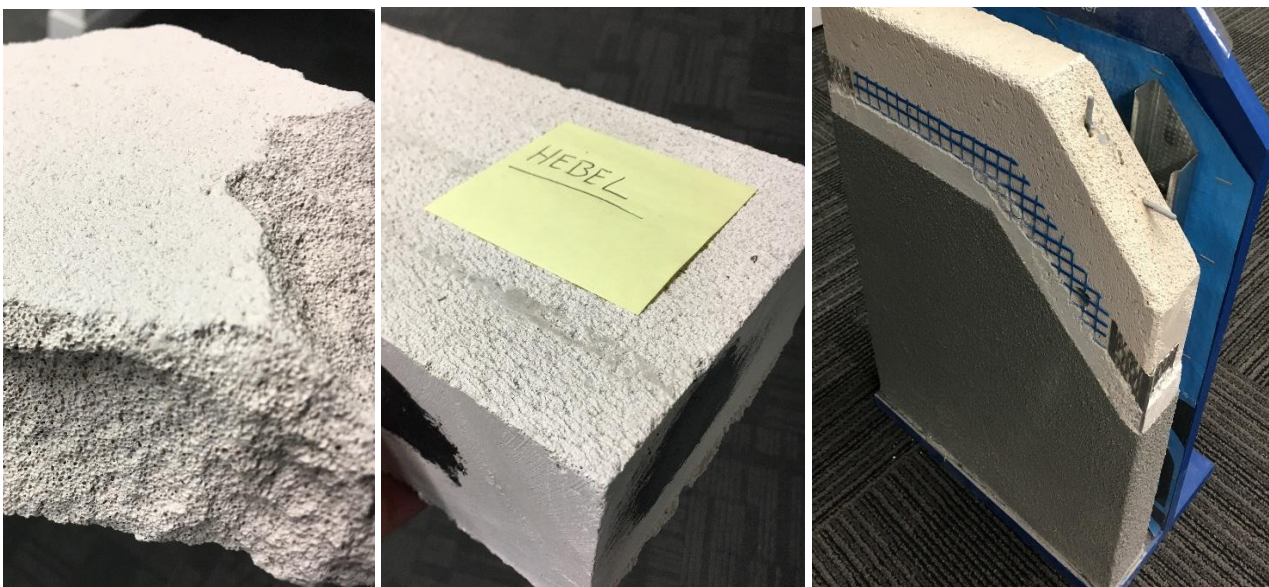
Figure 24. typical AAC structure (left), Hebel block (centre), Typical AAC EIFS installation (right), all photos by CSIRO.
