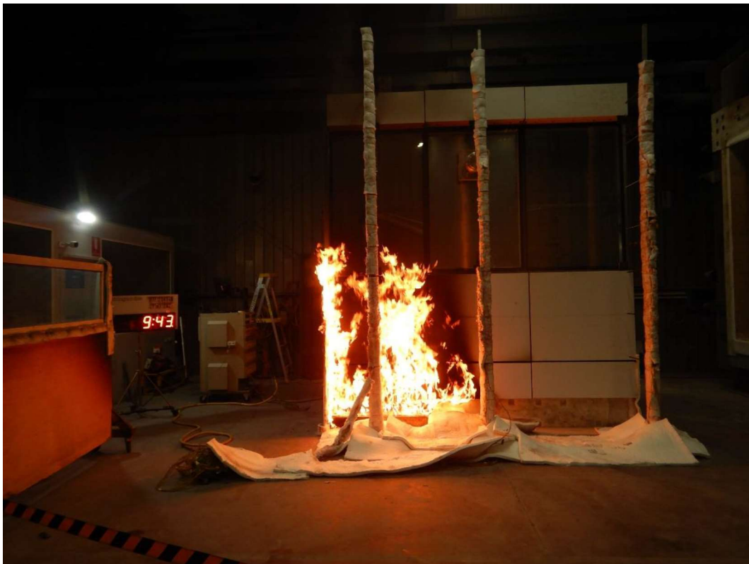
Figure 32 The specimen 9 minutes 43 seconds into the test (burner output at 300 kW)
