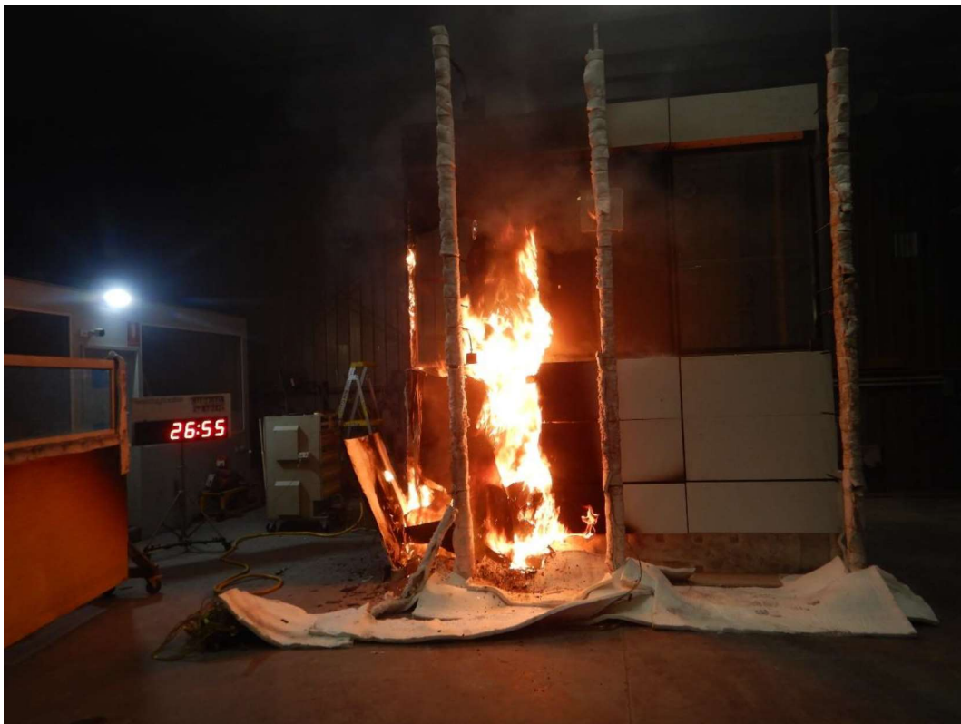
Figure 38 The specimen 26 minutes 55 seconds into the test (burner output at 300 kW)
