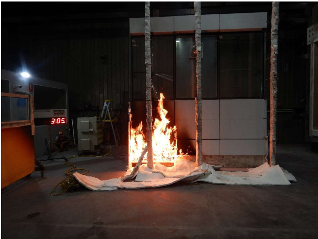
Figure 30 The specimen 3 minutes 5 seconds into the test (burner output at 300 kW)
