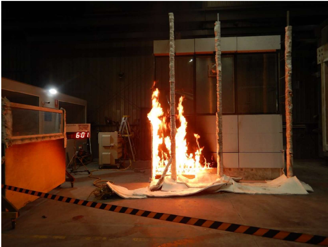
Figure 31 The specimen 6 minutes 1 second into the test (burner output at 300 kW)
