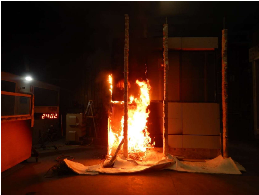
Figure 37 The specimen 24 minutes 2 seconds into the test (burner output at 300 kW)
