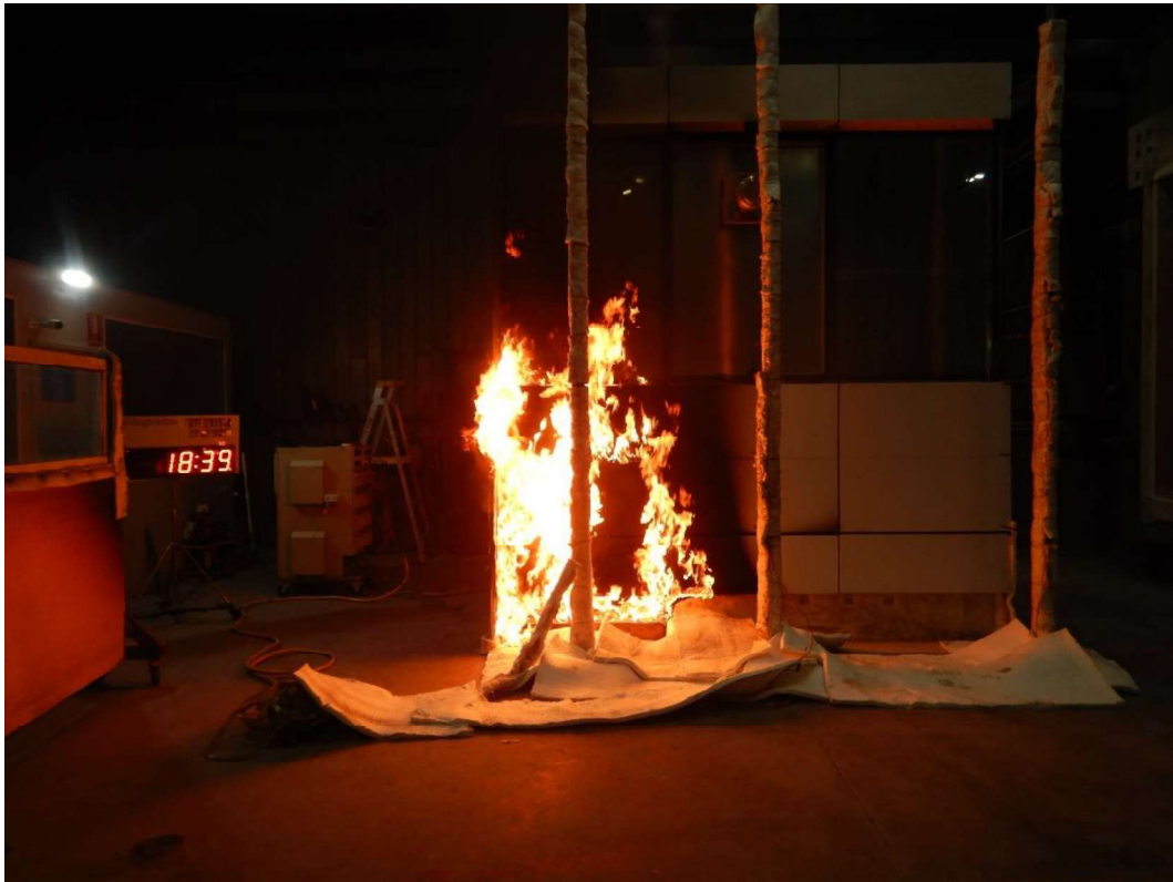
Figure 35 The specimen 18 minutes 39 seconds into the test (burner output at 300 kW)
