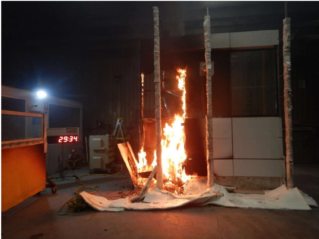
Figure 39 The specimen 29 minutes 34 seconds into the test (burner output at 300 kW)
