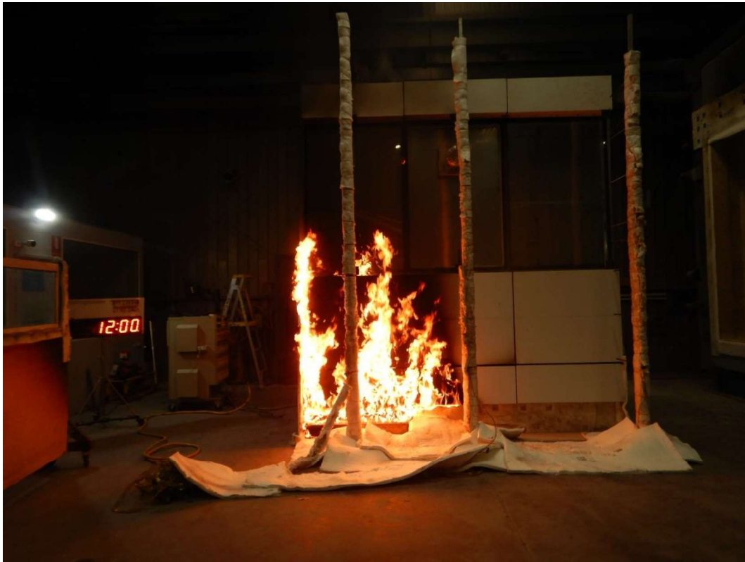
Figure 33 The specimen 12 minutes into the test (burner output at 300 kW)
