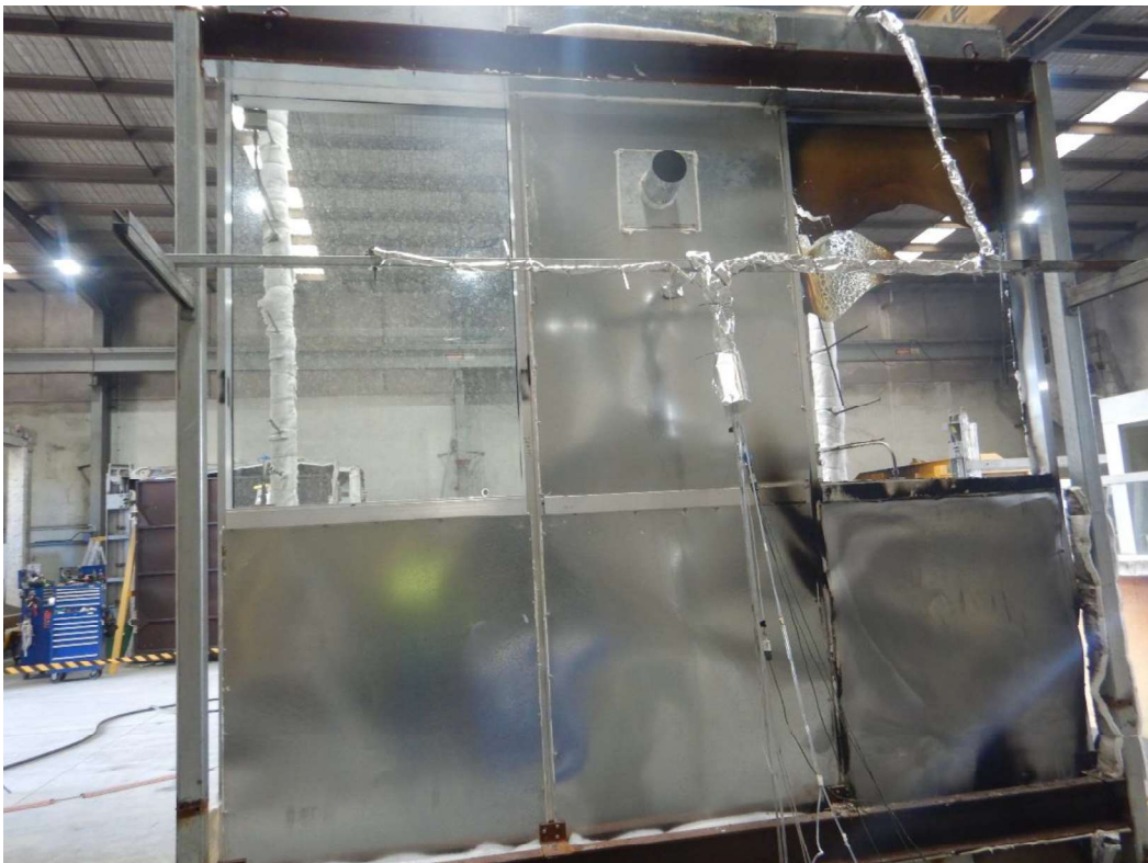
Figure 44 The specimen at end of test – unexposed side
