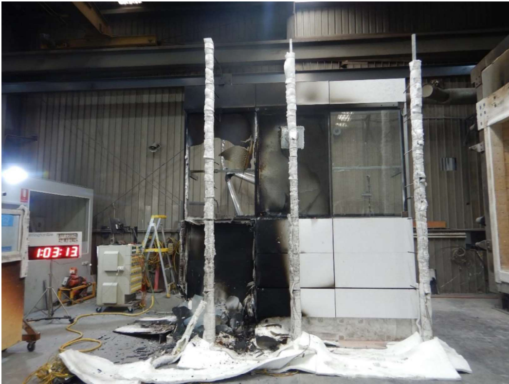
Figure 43 The specimen at end of test – exposed side
