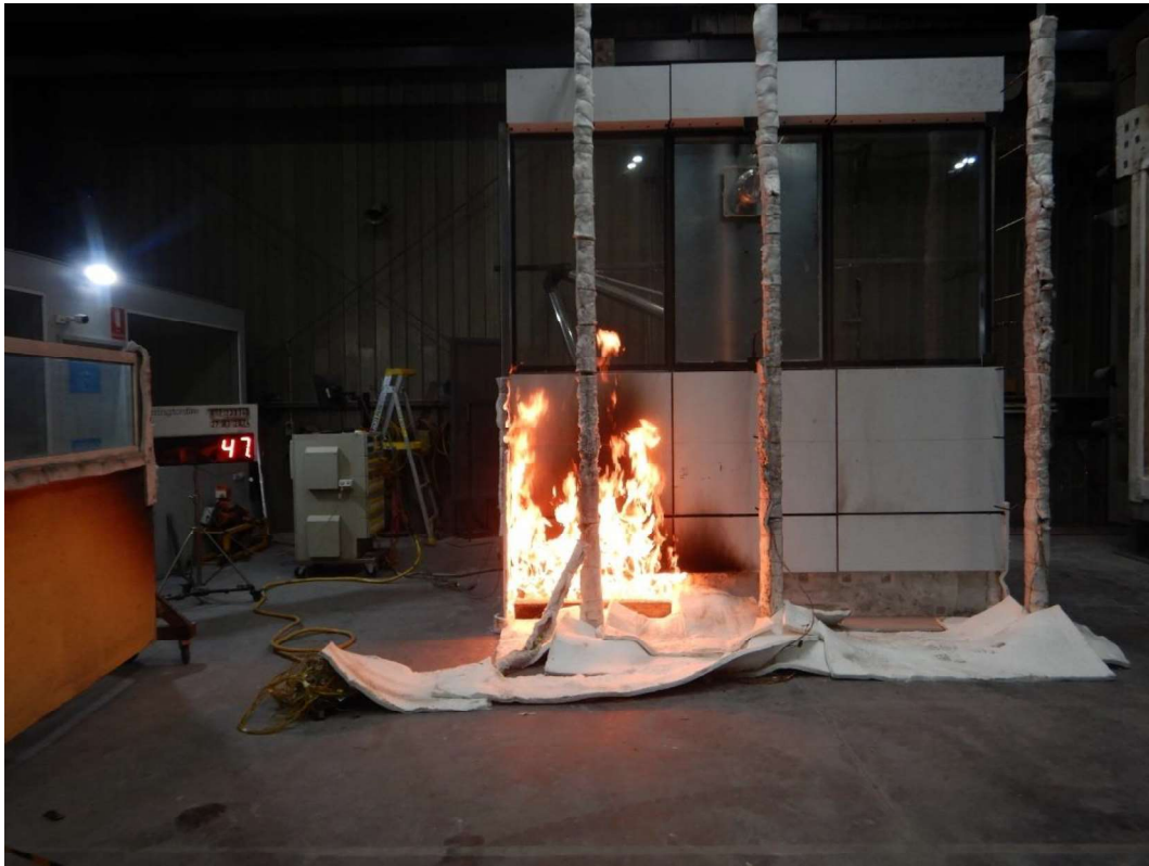
Figure 29 The specimen 47 seconds into the test (burner output at 300 kW)
