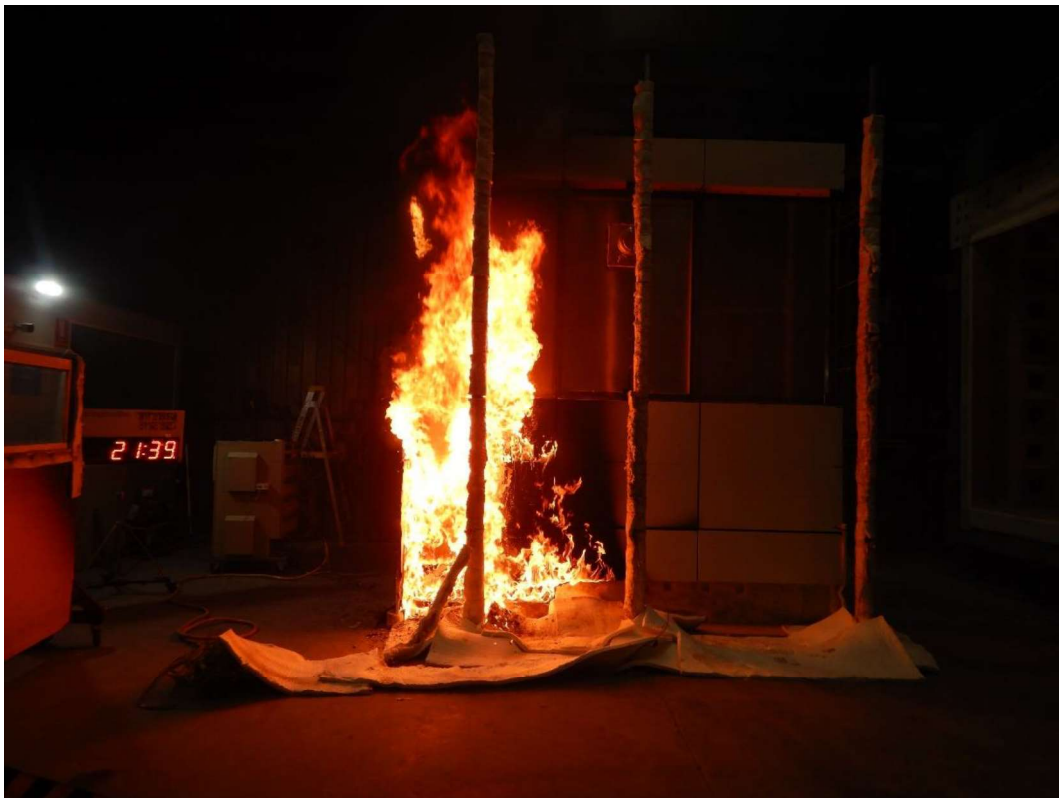
Figure 36 The specimen 21 minutes 39 seconds into the test (burner output at 300 kW)
