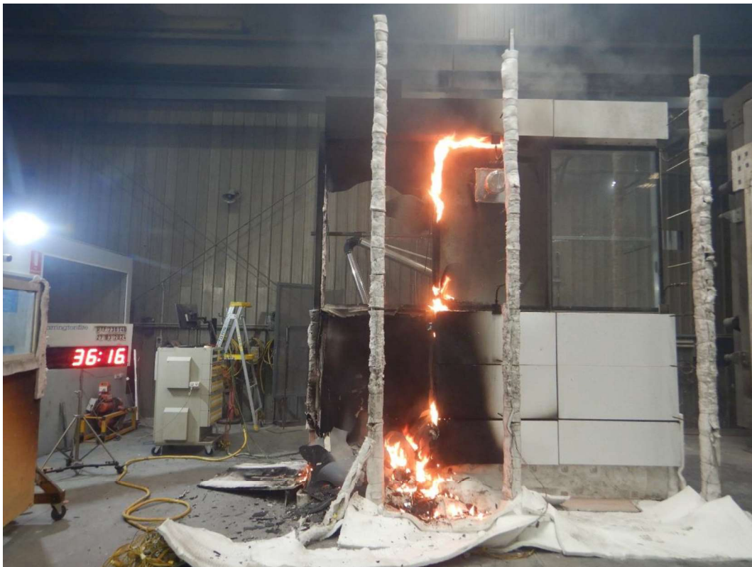
Figure 42 The specimen 36 minutes 16 seconds into the test (burner off)
