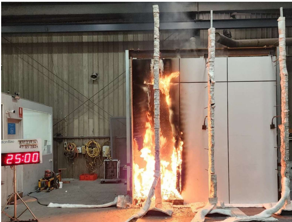
Figure 22 The specimen 25 minutes into the test (burner output at 300 kW).
