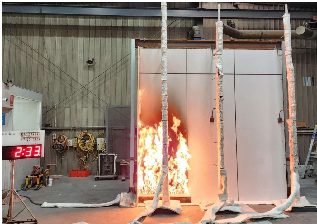
Figure 16 The specimen 2 minutes 33 seconds into the test (burner output at 300 kW)
