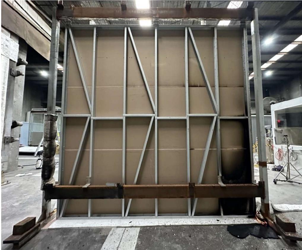
Figure 29 The unexposed side of the specimen at the end of test.
