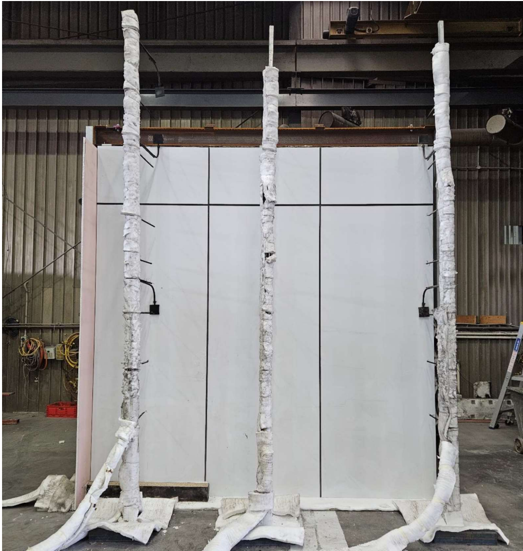
Figure 14 The specimen before the reaction to fire test - exposed side.
