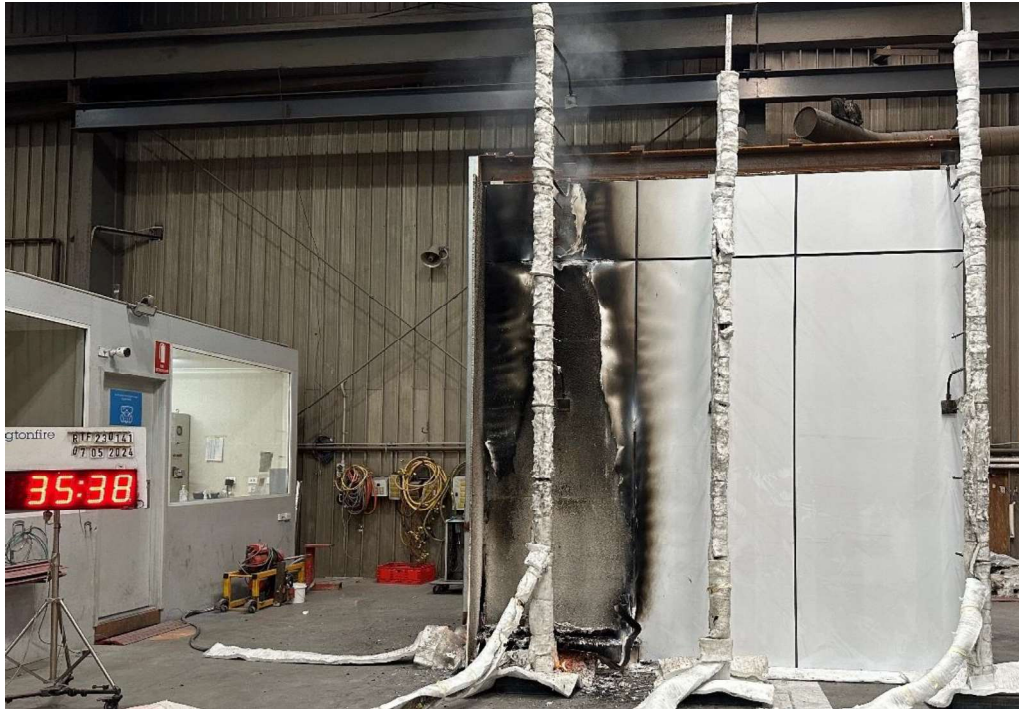
Figure 25 The specimen 35 minutes 38 seconds into the test (5 minutes 38 seconds after burner off).
