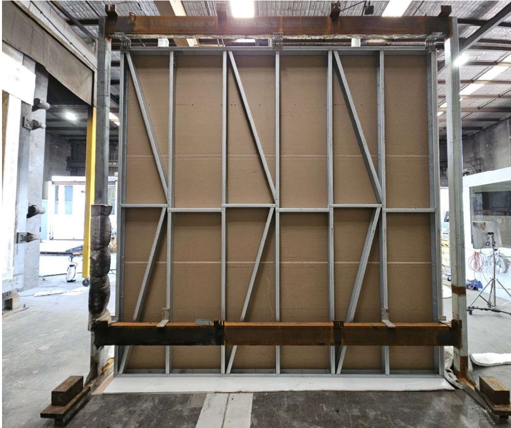
Figure 15 The specimen before the reaction to fire test - unexposed side.
