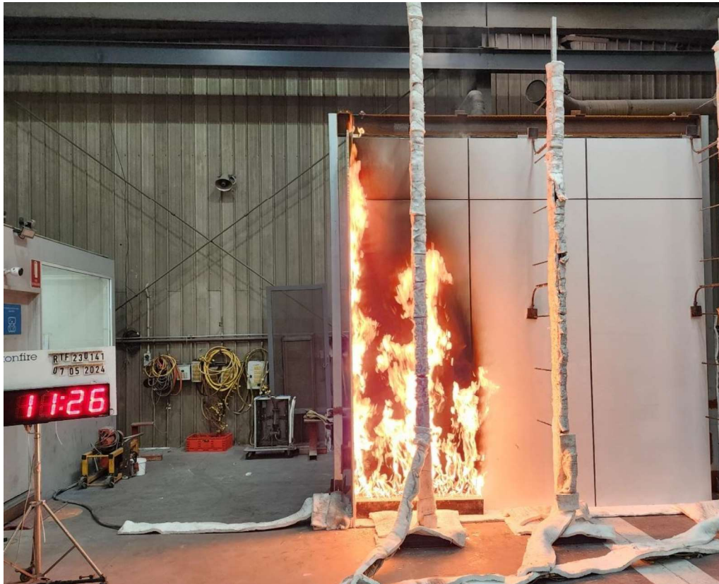
Figure 19 The specimen 11 minutes 26 seconds into the test (burner output at 300 kW)
