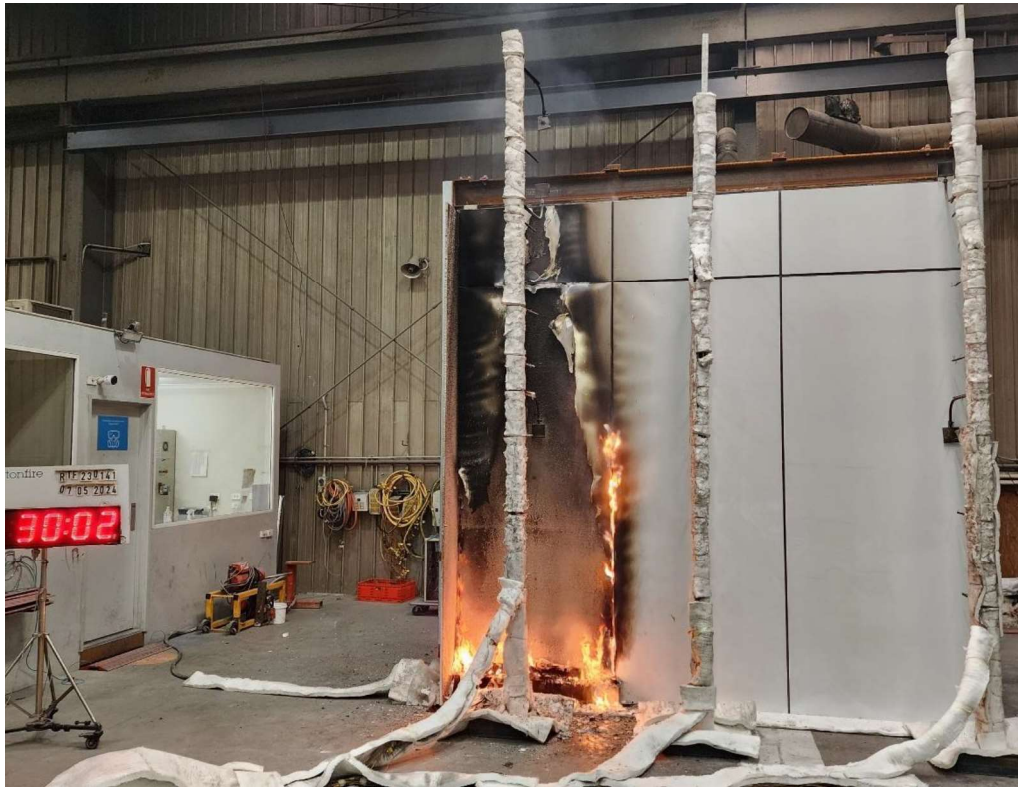
Figure 23 The specimen 30 minutes 2 seconds into the test (2 seconds after burner off).
