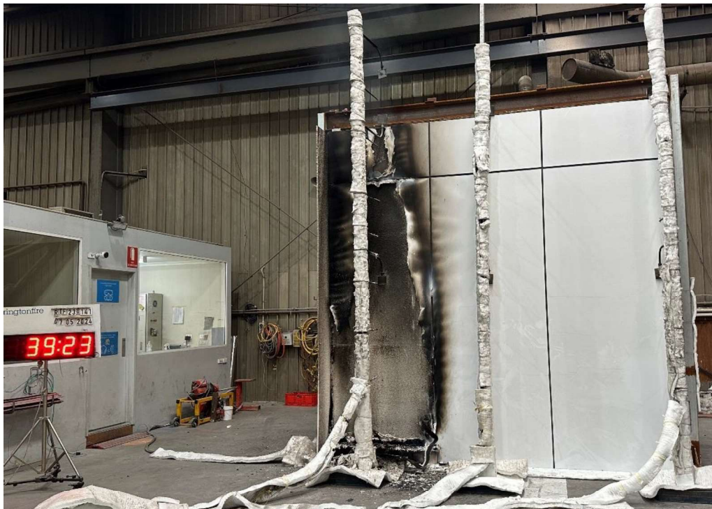
Figure 26 The specimen 39 minutes 23 seconds into the test (9 minutes 23 seconds after burner off).
