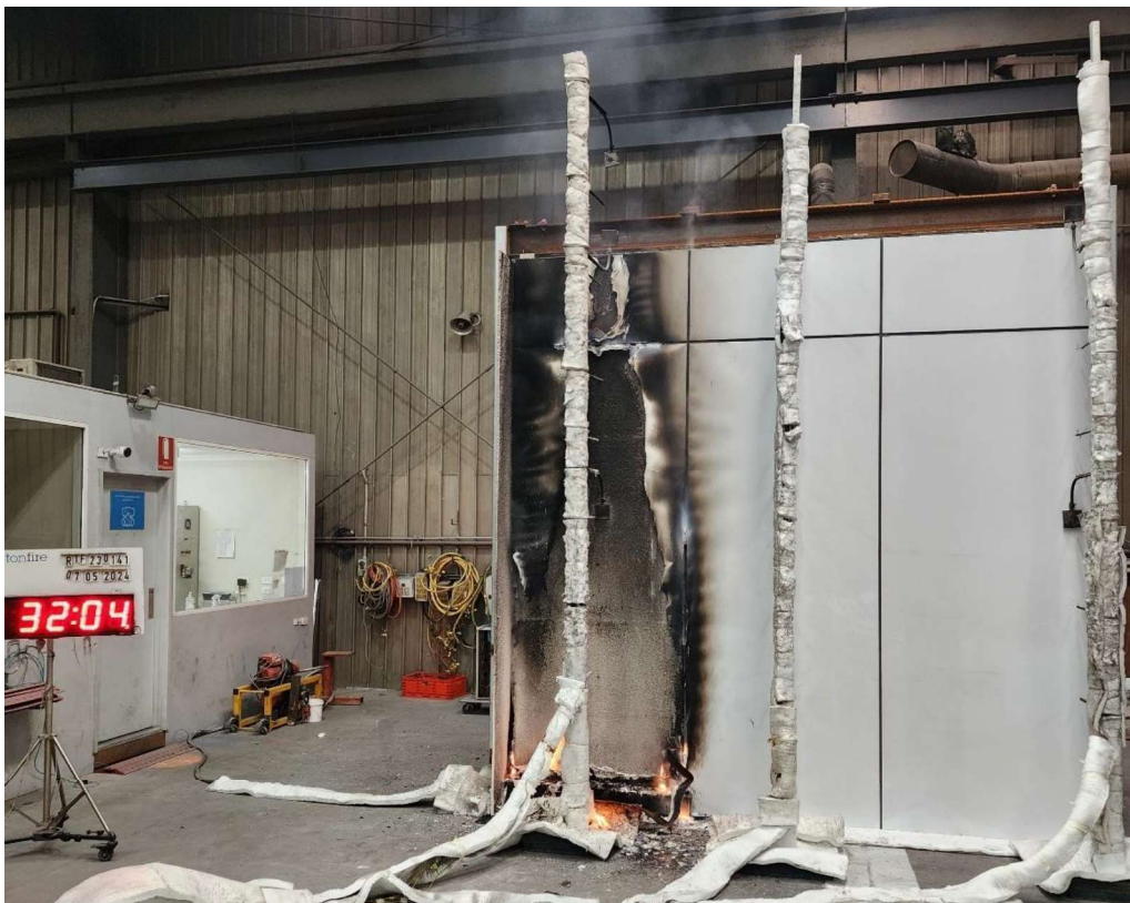
Figure 24 The specimen 32 minutes 4 seconds into the test (2 minutes 4 seconds after burner off).
