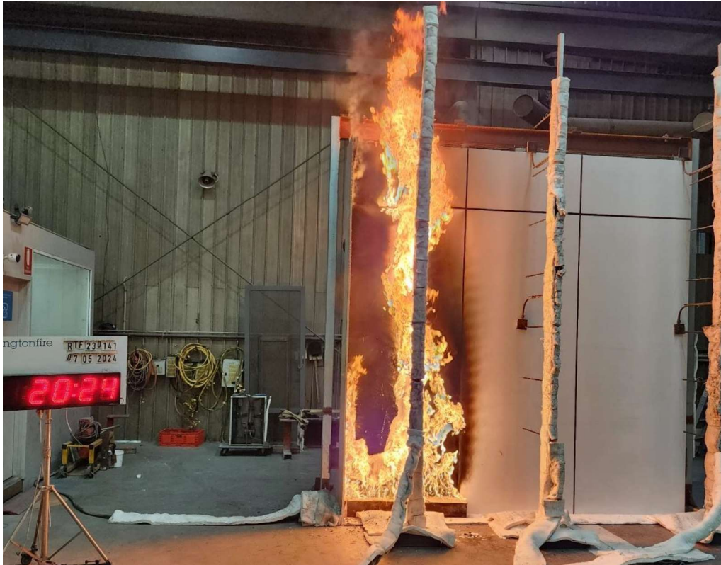
Figure 21 The specimen 20 minutes 24 seconds into the test (burner output at 300 kW).
