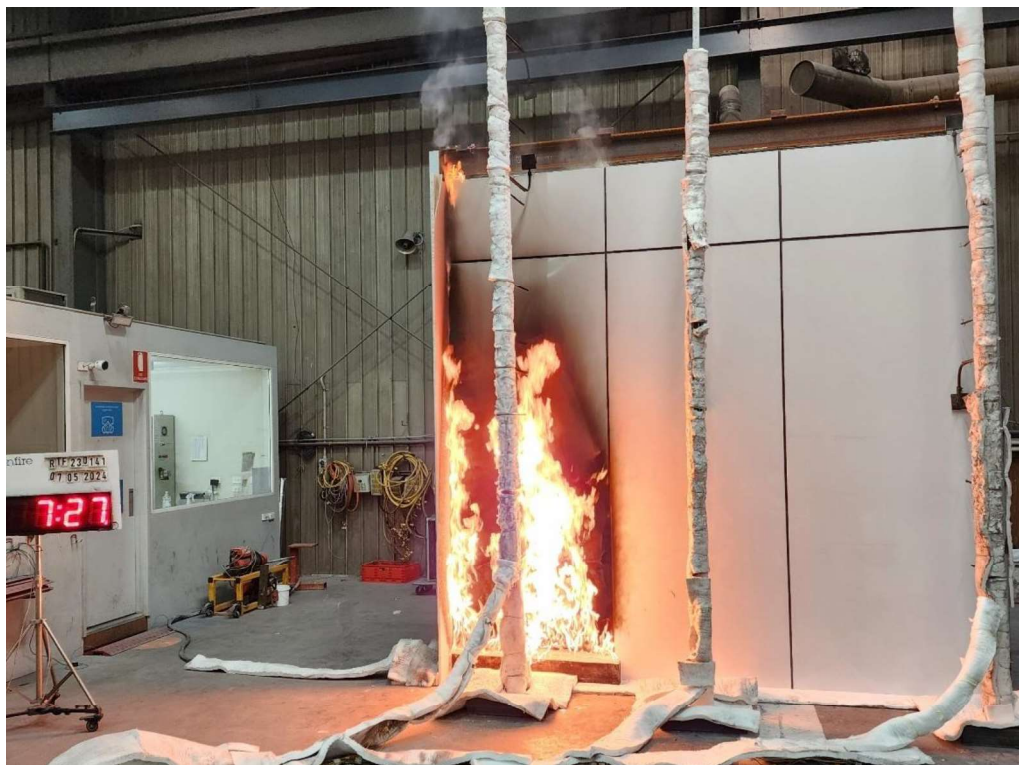
Figure 18 The specimen 7 minutes 27 seconds into the test (burner output at 300 kW)
