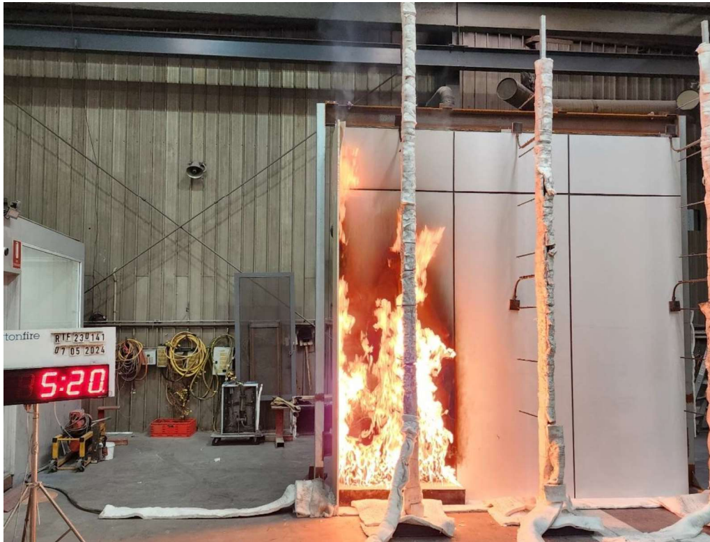
Figure 17 The specimen 5 minutes 20 seconds into the test (burner output at 300 kW)
