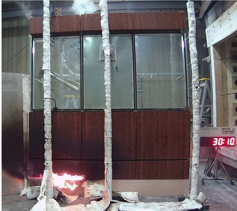
Figure 34 The specimen 30 minutes 10 seconds into the test (10 seconds after burner off and wind on).
