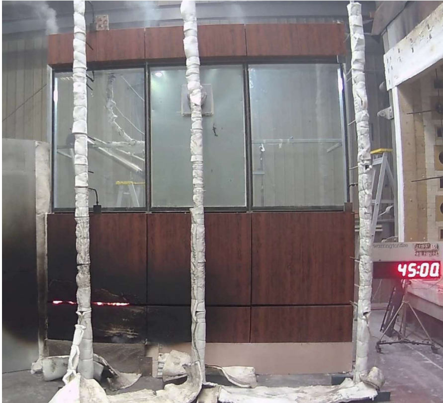
Figure 40 The specimen 45 minutes into the test (15 minutes after burner off and wind on).
