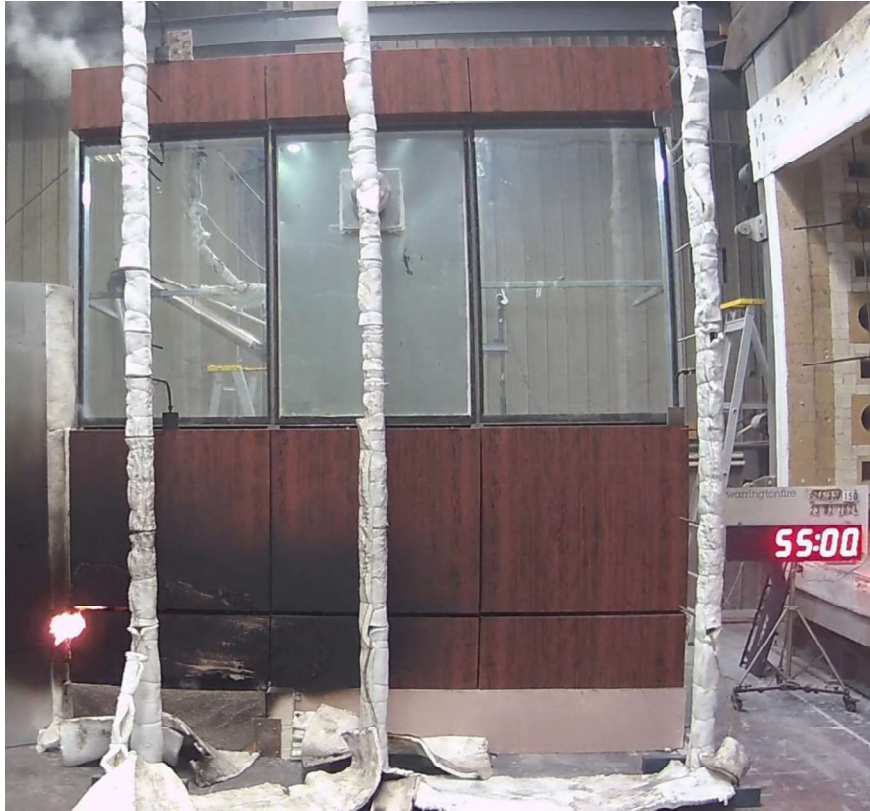
Figure 42 The specimen 55 minutes into the test (25 minutes after burner off and wind on).
