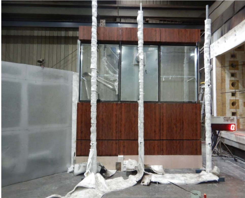
Figure 22 The specimen and test setup (angled - exposed side) before the reaction to fire test
