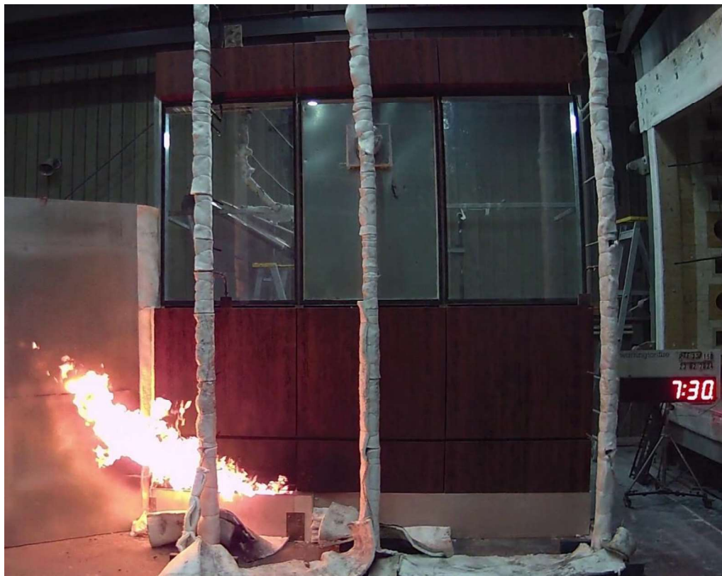
Figure 27 The specimen 7 minutes 30 seconds into the test (burner output at 300 kW and wind on)
