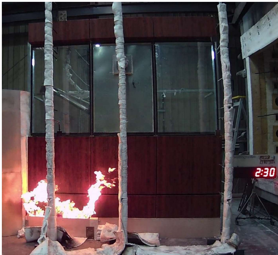
Figure 25 The specimen 2 minutes 30 seconds into the test (burner output at 300 kW and wind on)
