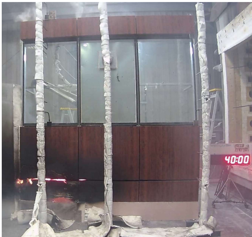
Figure 39 The specimen 40 minutes into the test (10 minutes after burner off and wind on).
