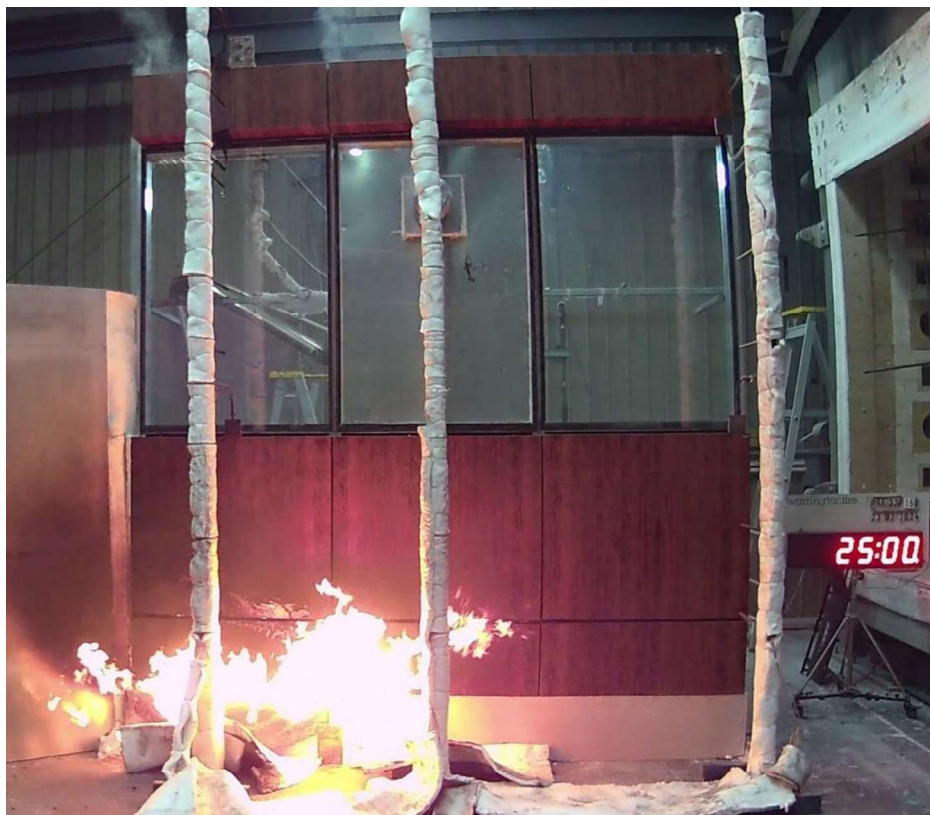
Figure 31 The specimen 25 minutes into the test (burner output at 300 kW and wind on).
