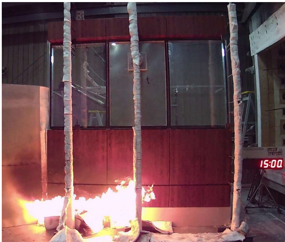
Figure 29 The specimen 15 minutes into the test (burner output at 300 kW and wind on).
