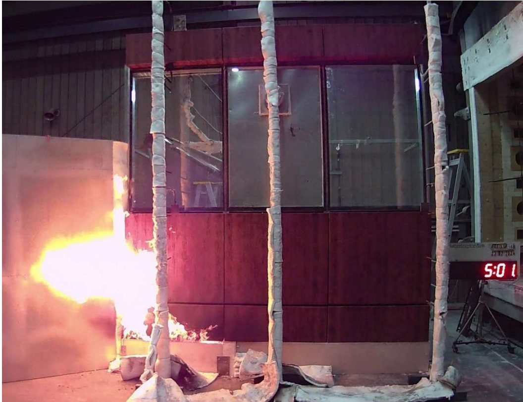
Figure 26 The specimen 5 minutes 1 second into the test (burner output at 300 kW and wind on)
