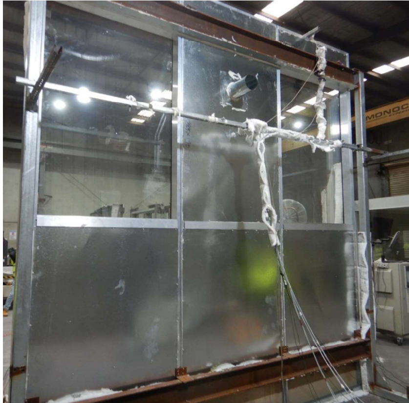
Figure 24 The specimen before the reaction to fire test - unexposed side.
