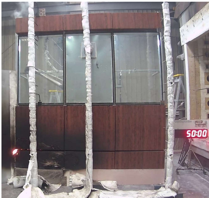
Figure 41 The specimen 50 minutes into the test (20 minutes after burner off and wind on).
