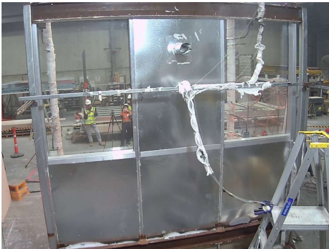
Figure 33 The unexposed side of the specimen 30 minutes into the test (burner off and wind on).
