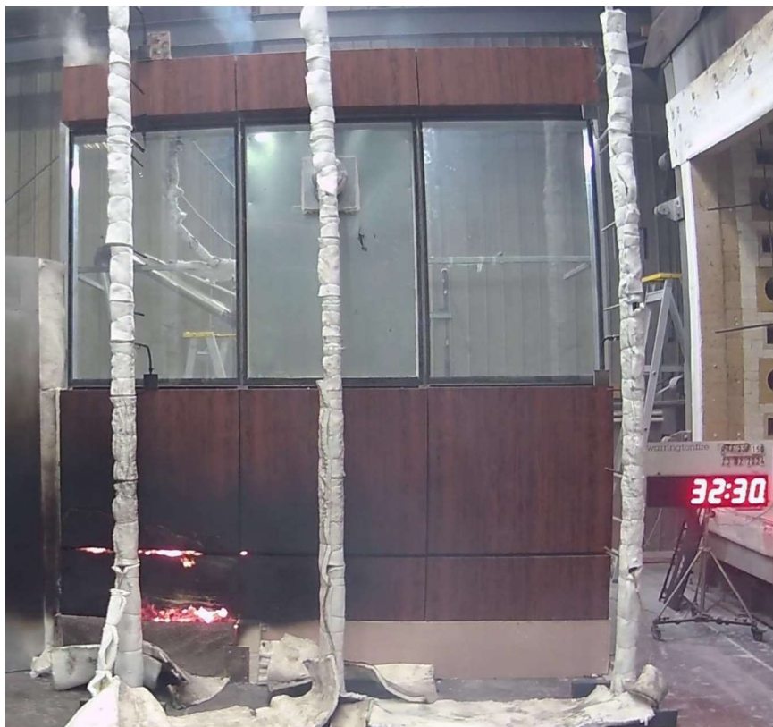
Figure 37 The specimen 32 minutes 30 seconds into the test (2 minutes 30 seconds after burner off and wind on).
