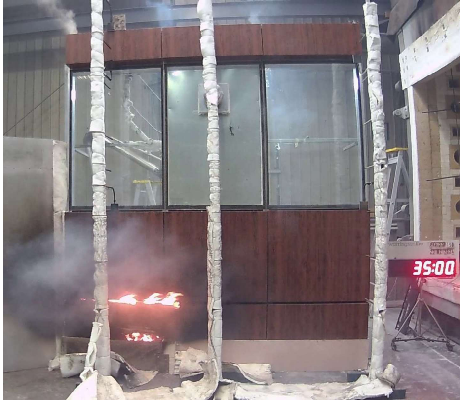
Figure 38 The specimen 35 minutes into the test (5 minutes after burner off and wind on).
