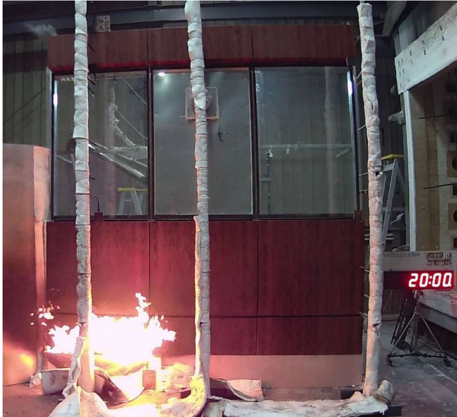
Figure 30 The specimen 20 minutes into the test (burner output at 300 kW and wind on).
