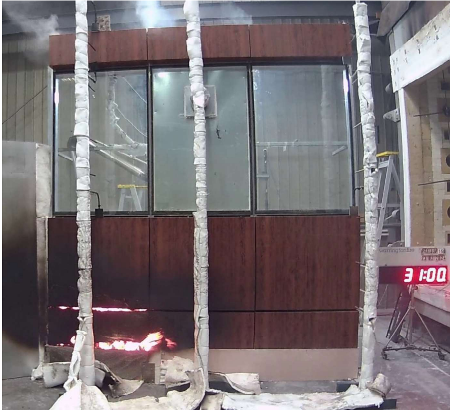
Figure 36 The specimen 31 minutes into the test (1minute after burner off and wind on).
