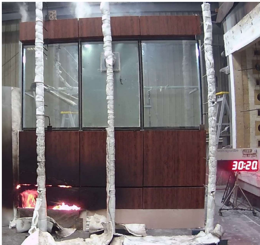
Figure 35 The specimen 30 minutes 20 seconds into the test (20 seconds after burner off and wind on).
