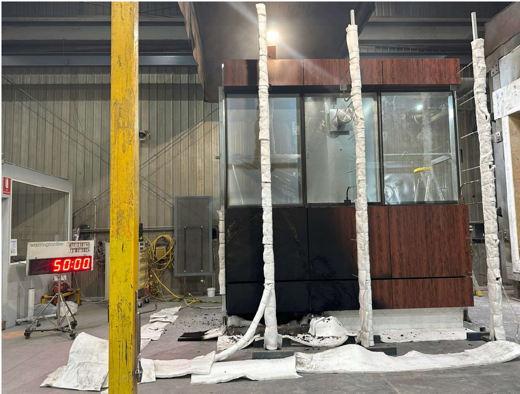
Figure 39 The specimen 50 minutes into the test (burner off)
