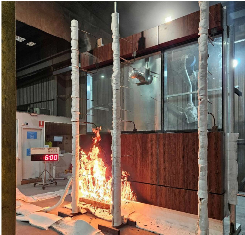
Figure 31 The specimen 6 minutes into the test (burner output at 300 kW)
