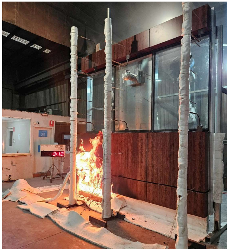
Figure 30 The specimen 3 minutes 12 seconds into the test (burner output at 300 kW)
