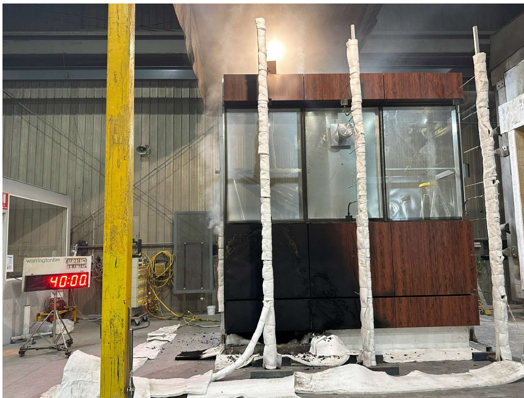
Figure 38 The specimen 40 minutes into the test (burner off)
