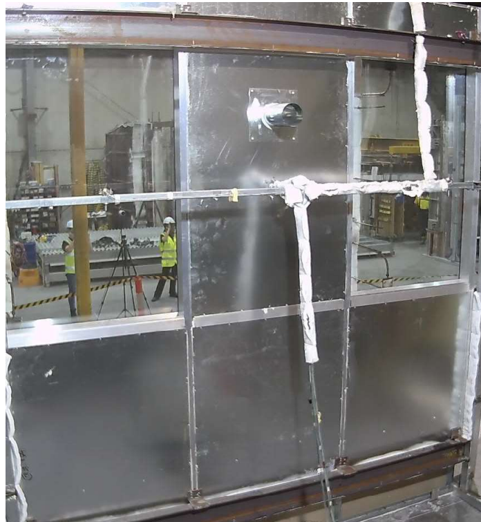
Figure 28 The specimen (unexposed side) before the reaction to fire test
