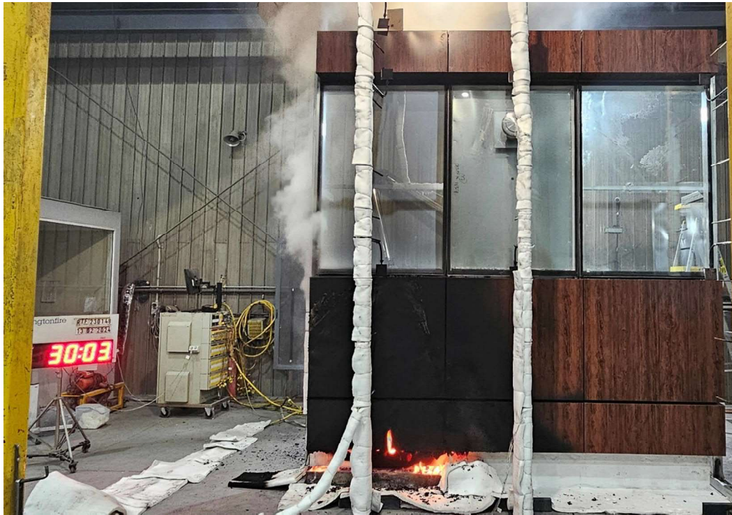
Figure 37 The specimen 30 minutes 3 seconds into the test (burner off)
