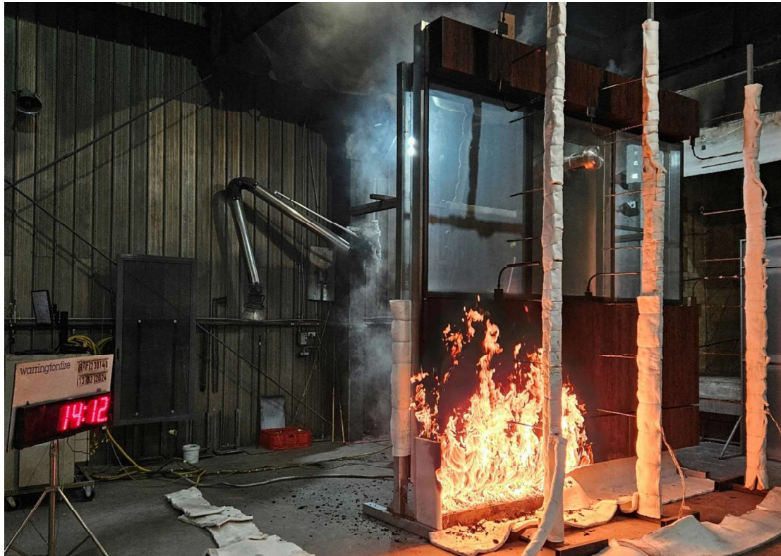
Figure 33 The specimen 14 minutes 12 seconds into the test (burner output at 300 kW)
