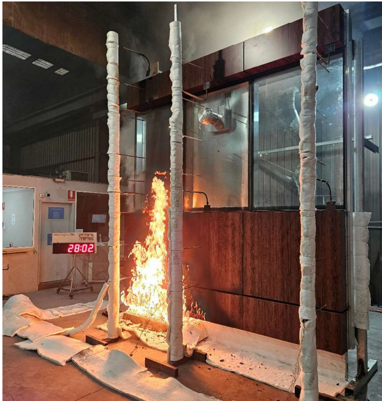
Figure 35 The specimen 28 minutes 2 seconds into the test (burner output at 300 kW)
