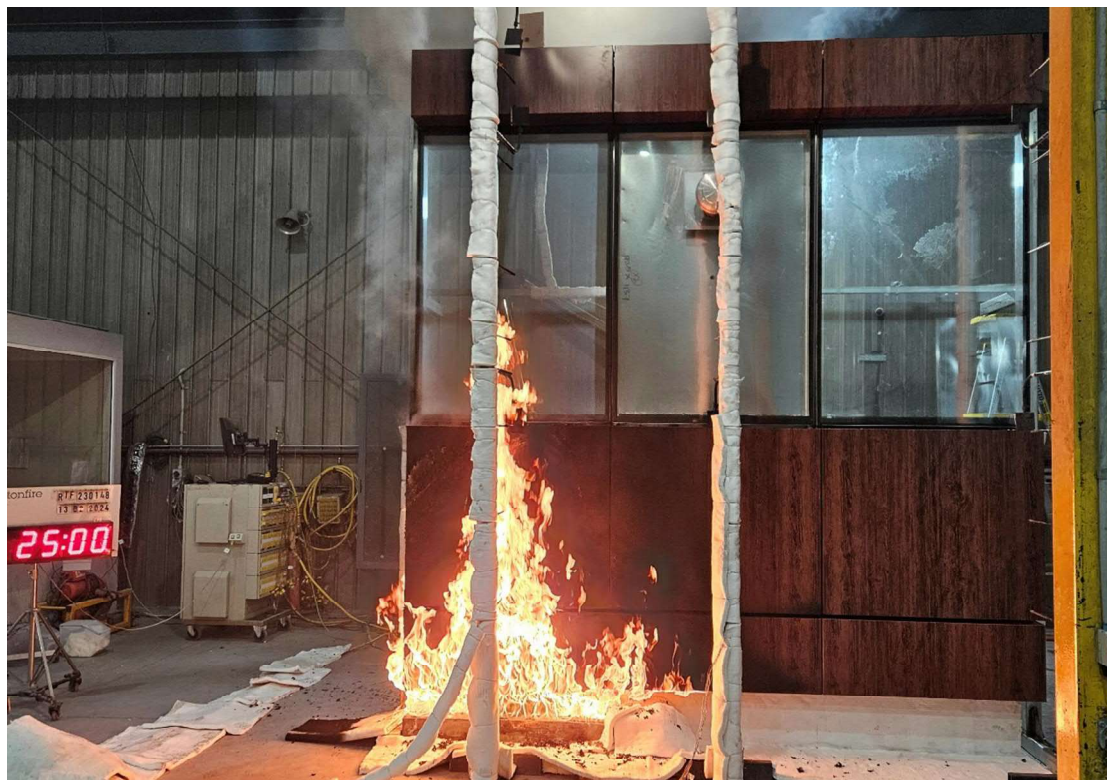
Figure 34 The specimen 25 minutes into the test (burner output at 300 kW)
