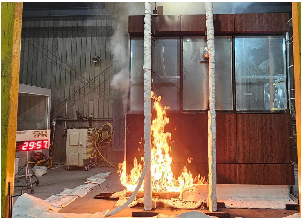
Figure 36 The specimen 29 minutes 57 seconds into the test (burner output at 300 kW)
