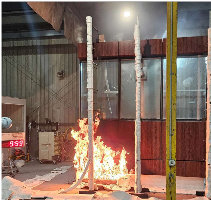
Figure 32 The specimen 9 minutes 59 seconds into the test (burner output at 300 kW)
