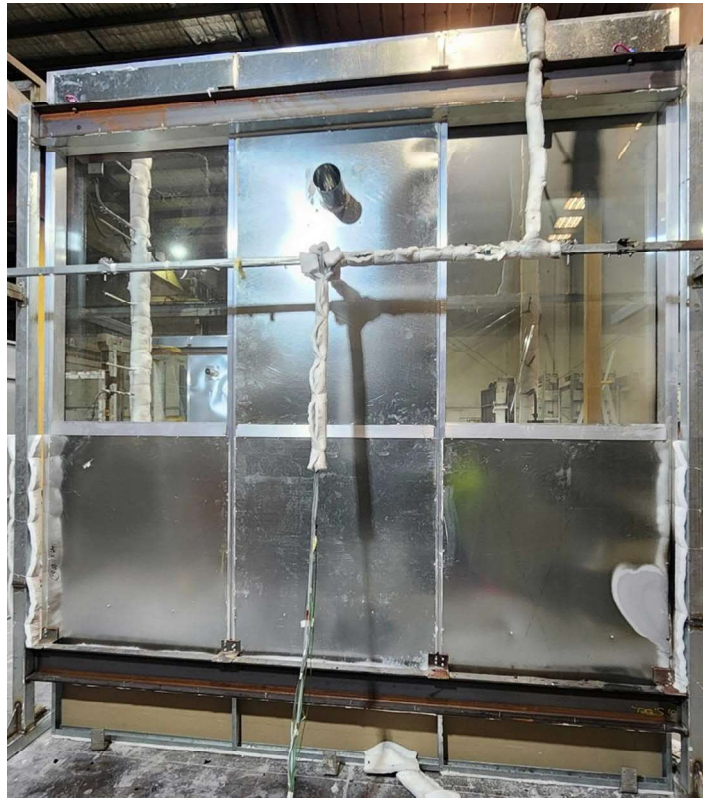
Figure 41 The specimen at end of test – unexposed side
