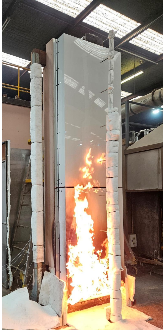
Figure 14 The specimen 3 minutes into the test (burner output at 200 kW)
