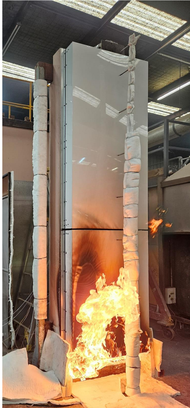
Figure 15 The specimen 4 minutes into the test (burner output at 200 kW)
