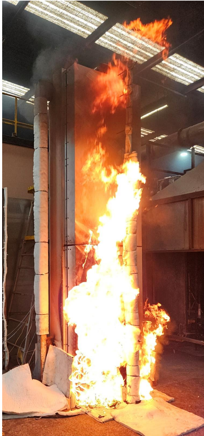
Figure 17 The specimen 6 minutes into the test (burner output at 200 kW)
