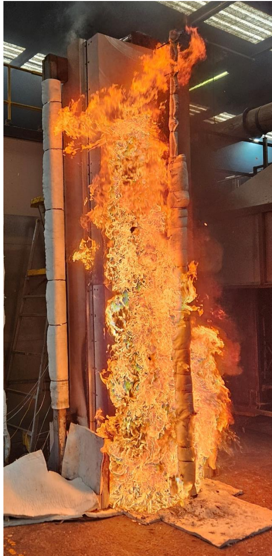
Figure 19 The specimen 6 minutes 22 seconds into the test (burner output at 200 kW)
