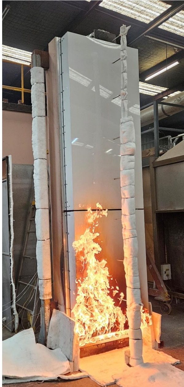
Figure 13 The specimen 2 minutes into the test (burner output at 200 kW)
