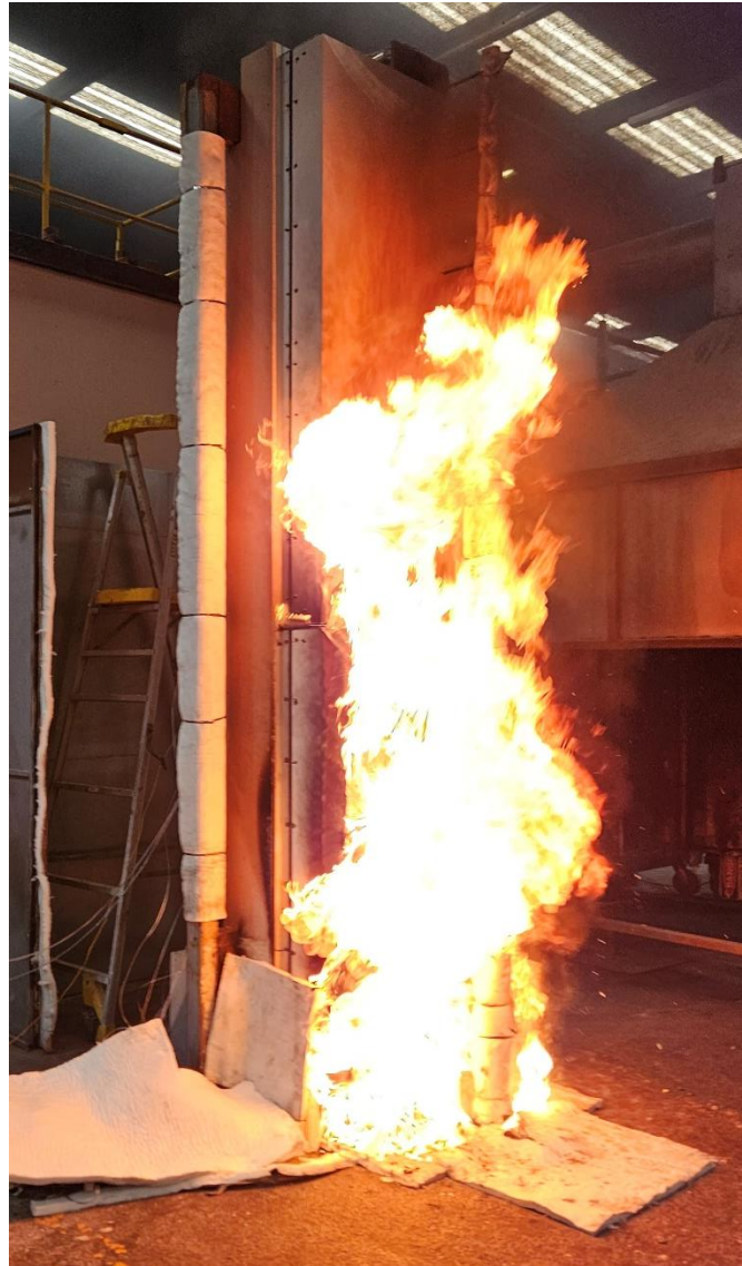
Figure 18 The specimen 6 minutes 17 seconds into the test (burner output at 200 kW)
