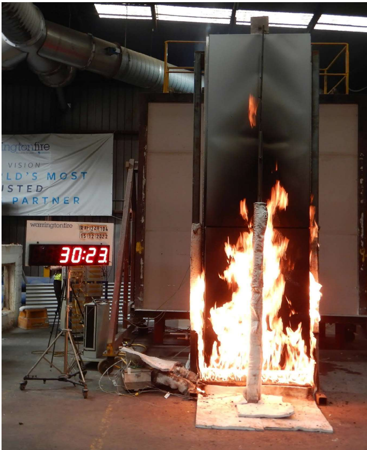
Figure 14 The specimen 30 minutes 23 seconds into the test (15 minutes 23 seconds after burner output was increased to 300 kW)
