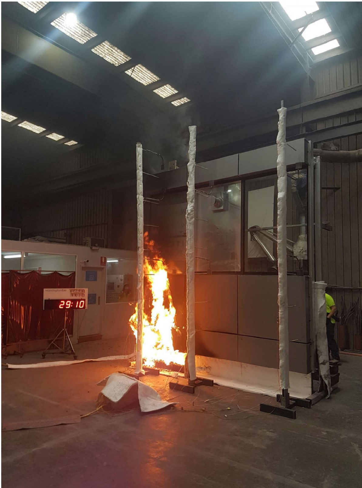
Figure 50 The specimen 29 minutes 10 seconds into the test (burner output at 300 kW)
