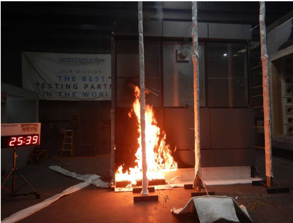
Figure 45 The specimen 25 minutes 39 seconds into the test (burner output at 300 kW)
