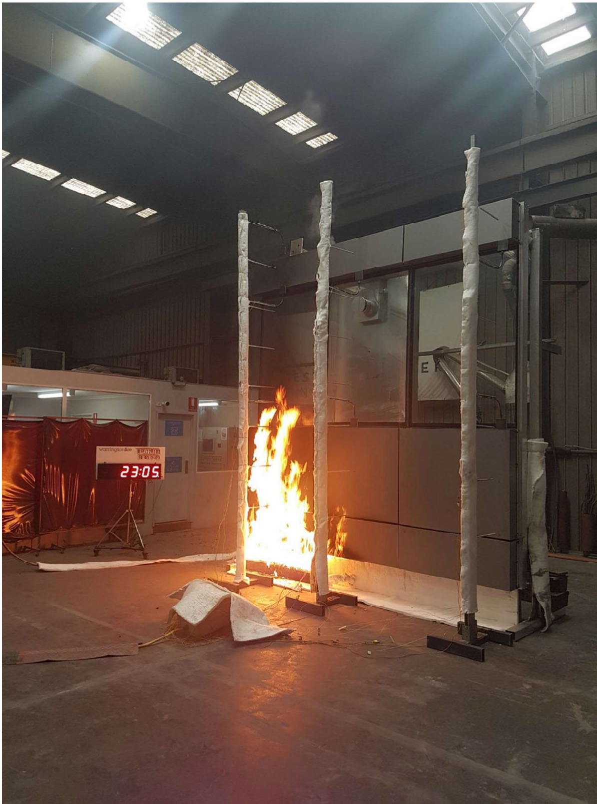
Figure 42 The specimen 23 minutes 5 seconds into the test (burner output at 300 kW)
