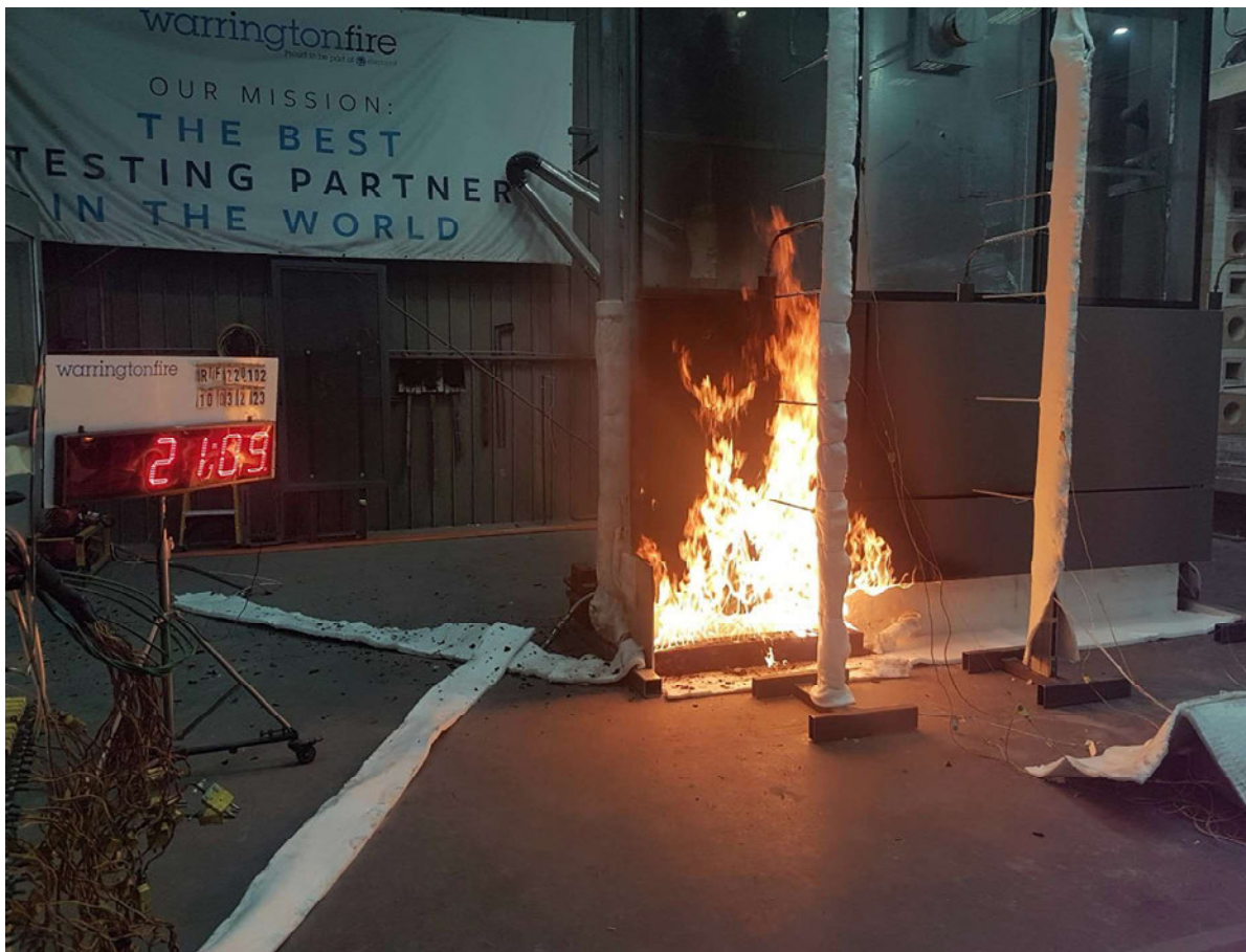
Figure 39 The specimen 21 minutes 9 seconds into the test (burner output at 300 kW)
