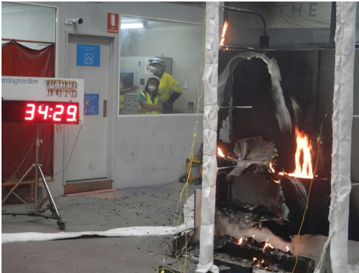
Figure 55 The specimen 34 minutes 29 seconds into the test (burner off).
