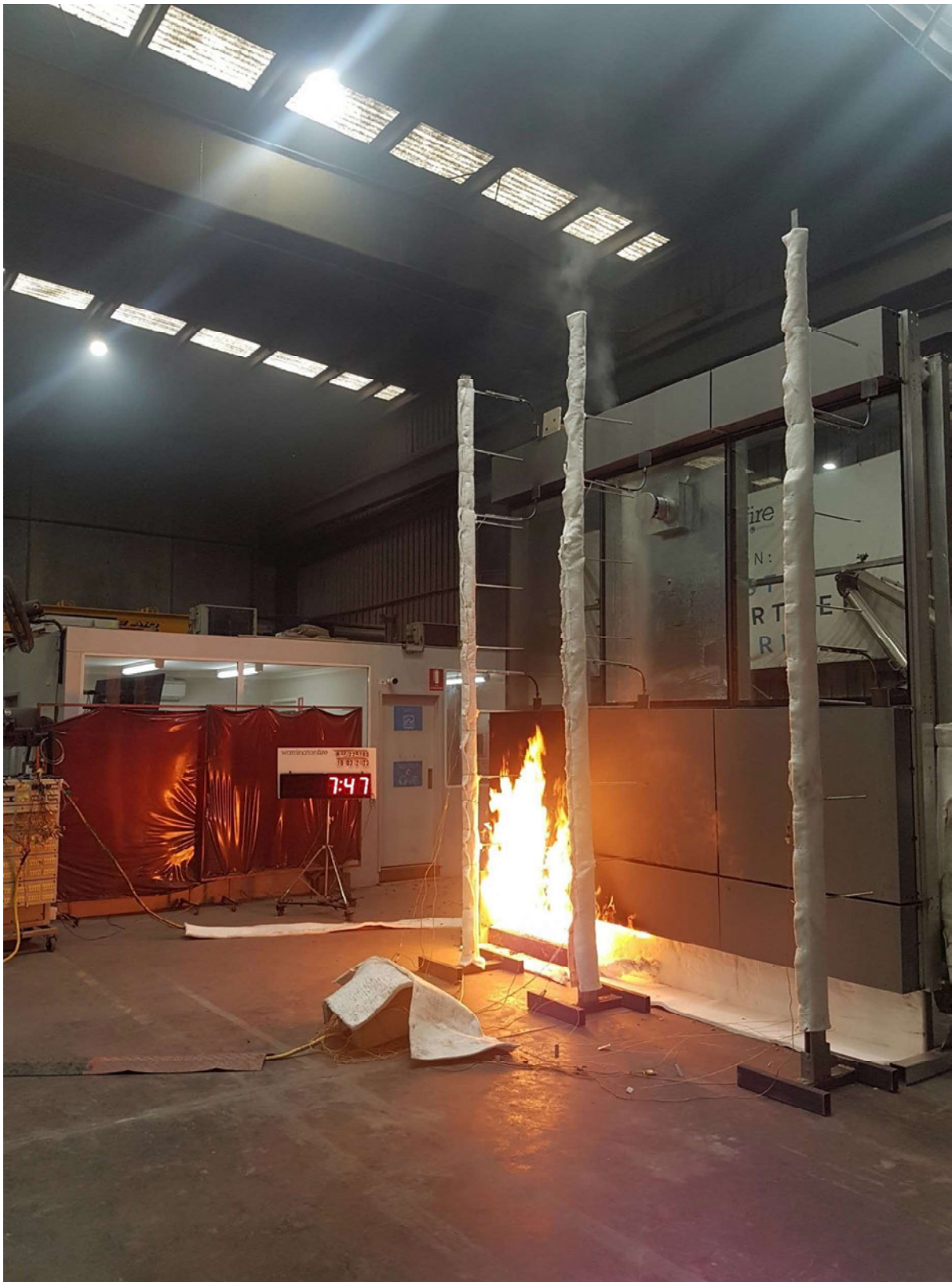
Figure 28 The specimen 7 minutes 47 seconds into the test (burner output at 300 kW)
