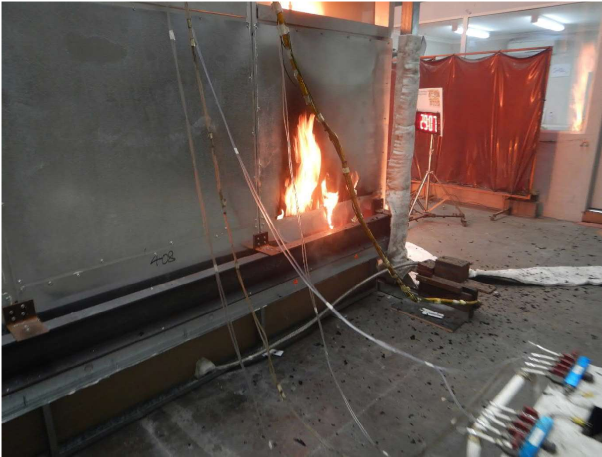
Figure 49 The specimen 29 minutes 7 seconds into the test (burner output at 300 kW) – unexposed side.
