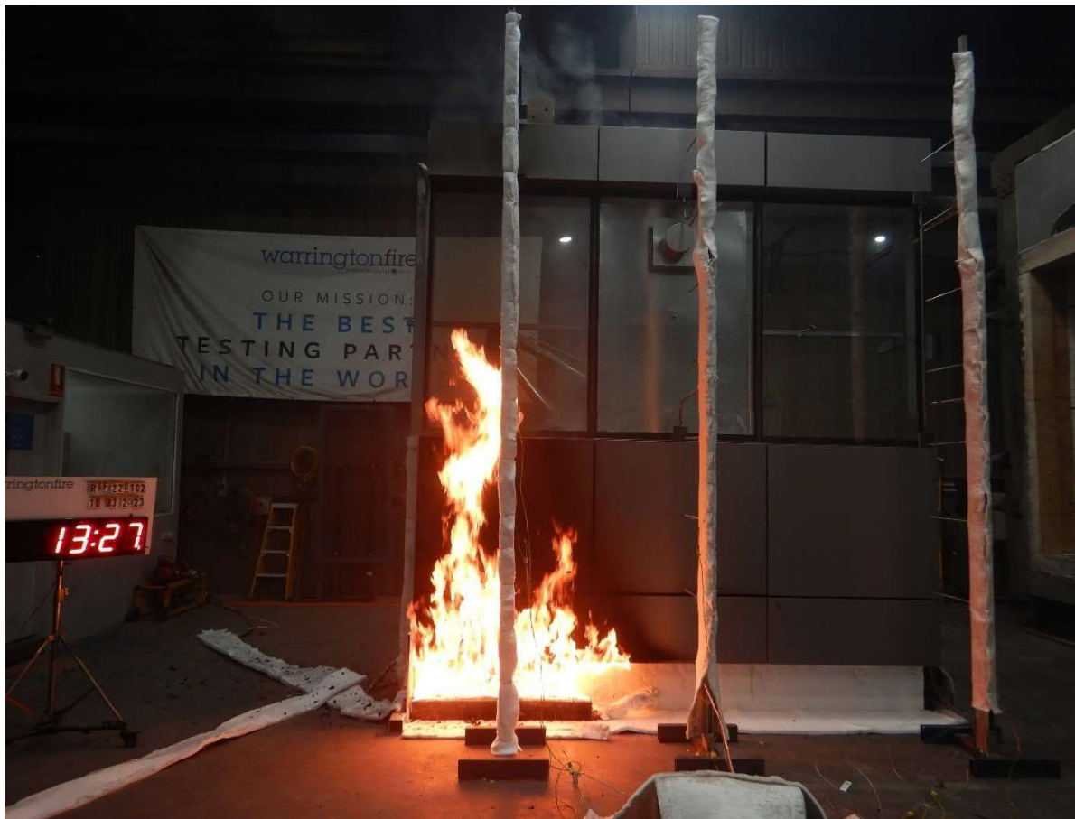
Figure 32 The specimen 13 minutes 27 seconds into the test (burner output at 300 kW)
