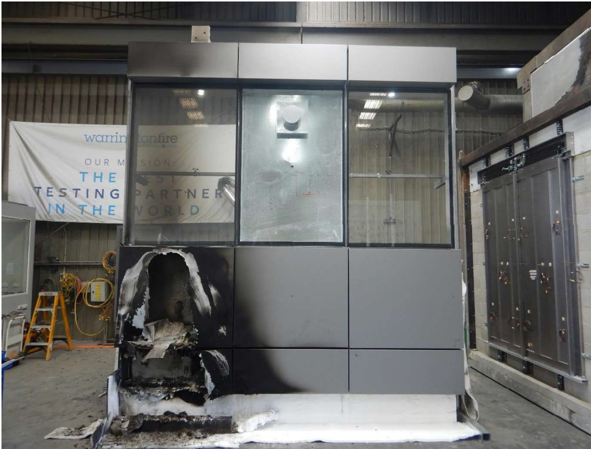
Figure 60 The specimen at end of test – exposed side.
