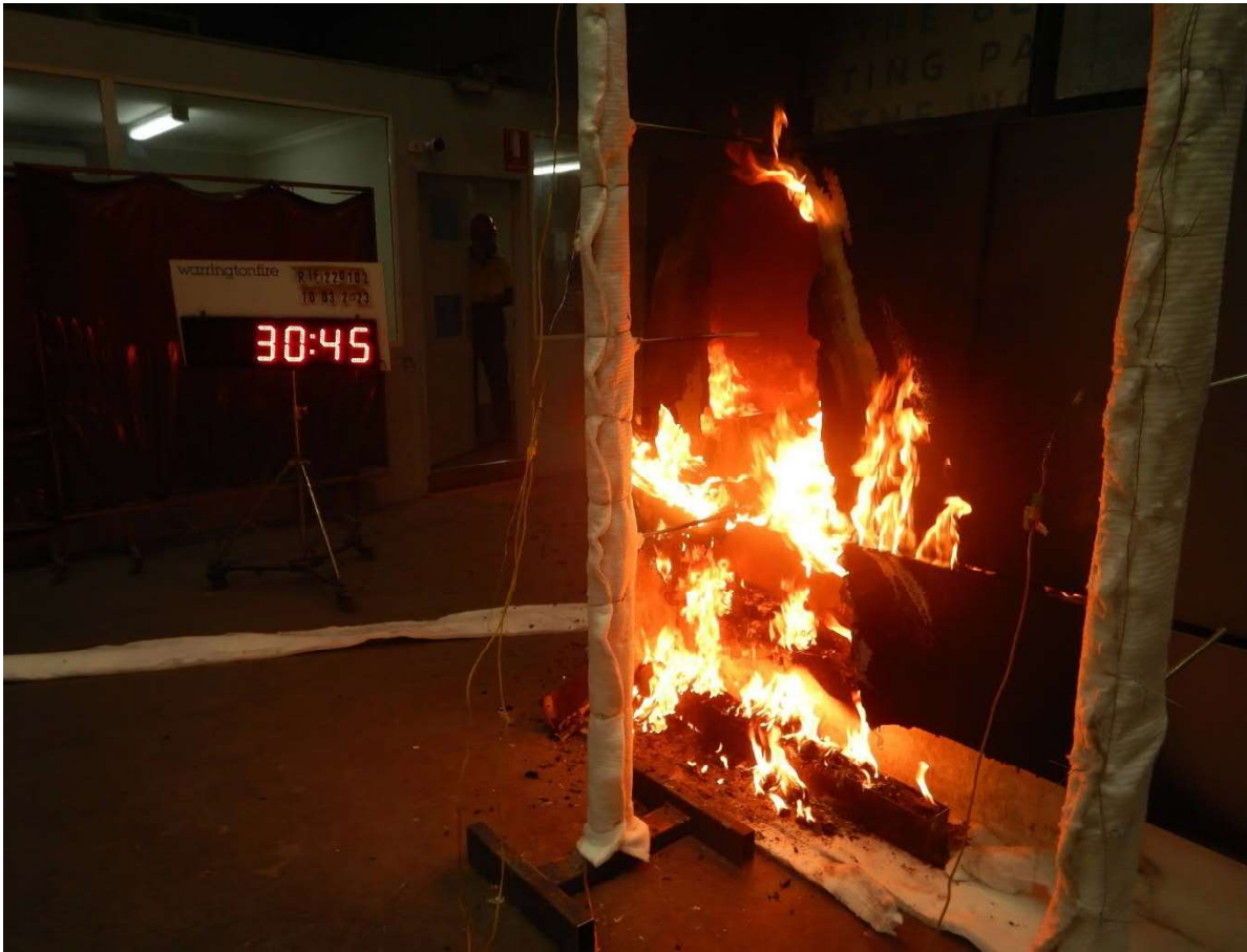
Figure 53 The specimen 30 minutes 45 seconds into the test (burner off).
