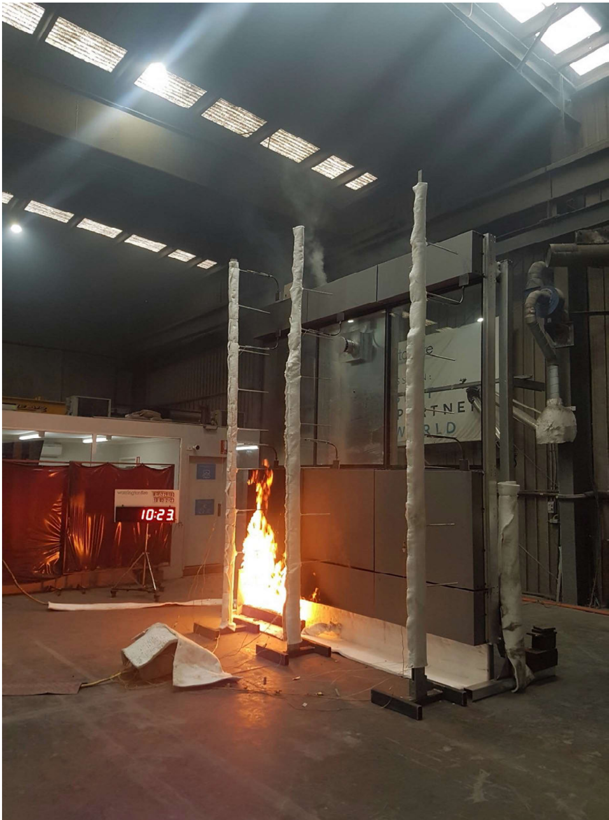
Figure 30 The specimen 10 minutes 23 seconds into the test (burner output at 300 kW)
