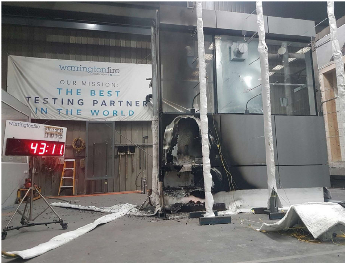
Figure 59 The specimen 43 minutes 11 seconds into the test (burner off).
