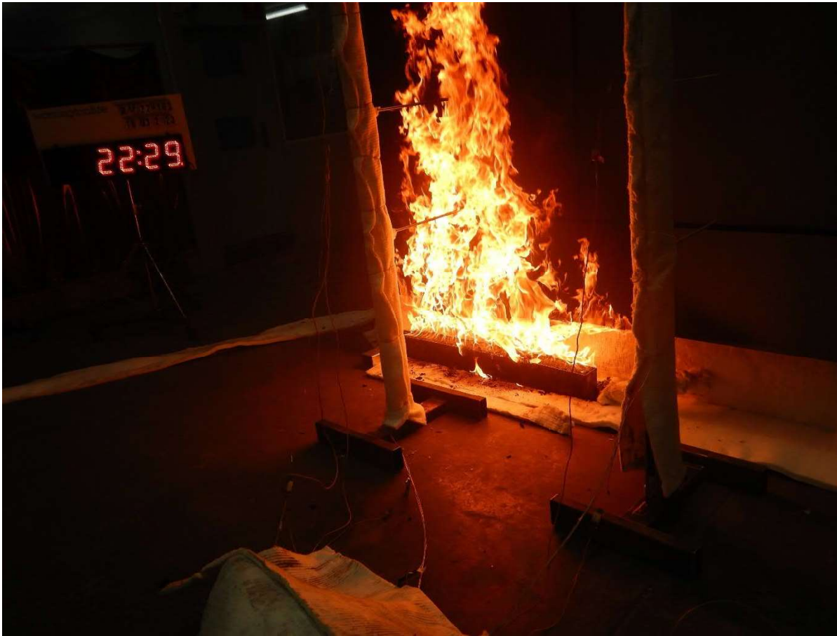
Figure 41 The specimen 22 minutes 29 seconds into the test (burner output at 300 kW)
