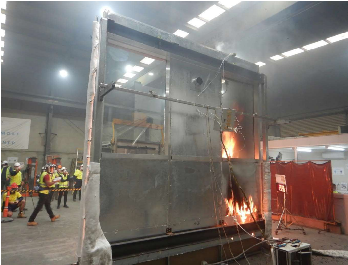
Figure 51 The specimen 29 minutes 38 seconds into the test (burner output at 300 kW) – unexposed side.
