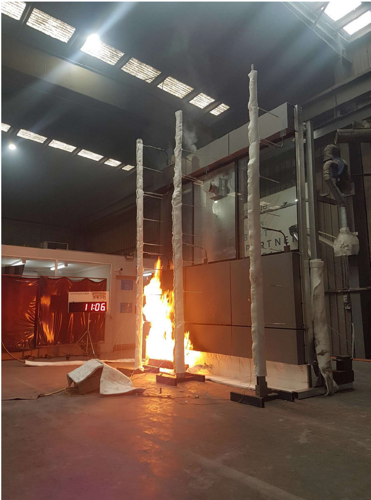
Figure 31 The specimen 11 minutes 6 seconds into the test (burner output at 300 kW)
