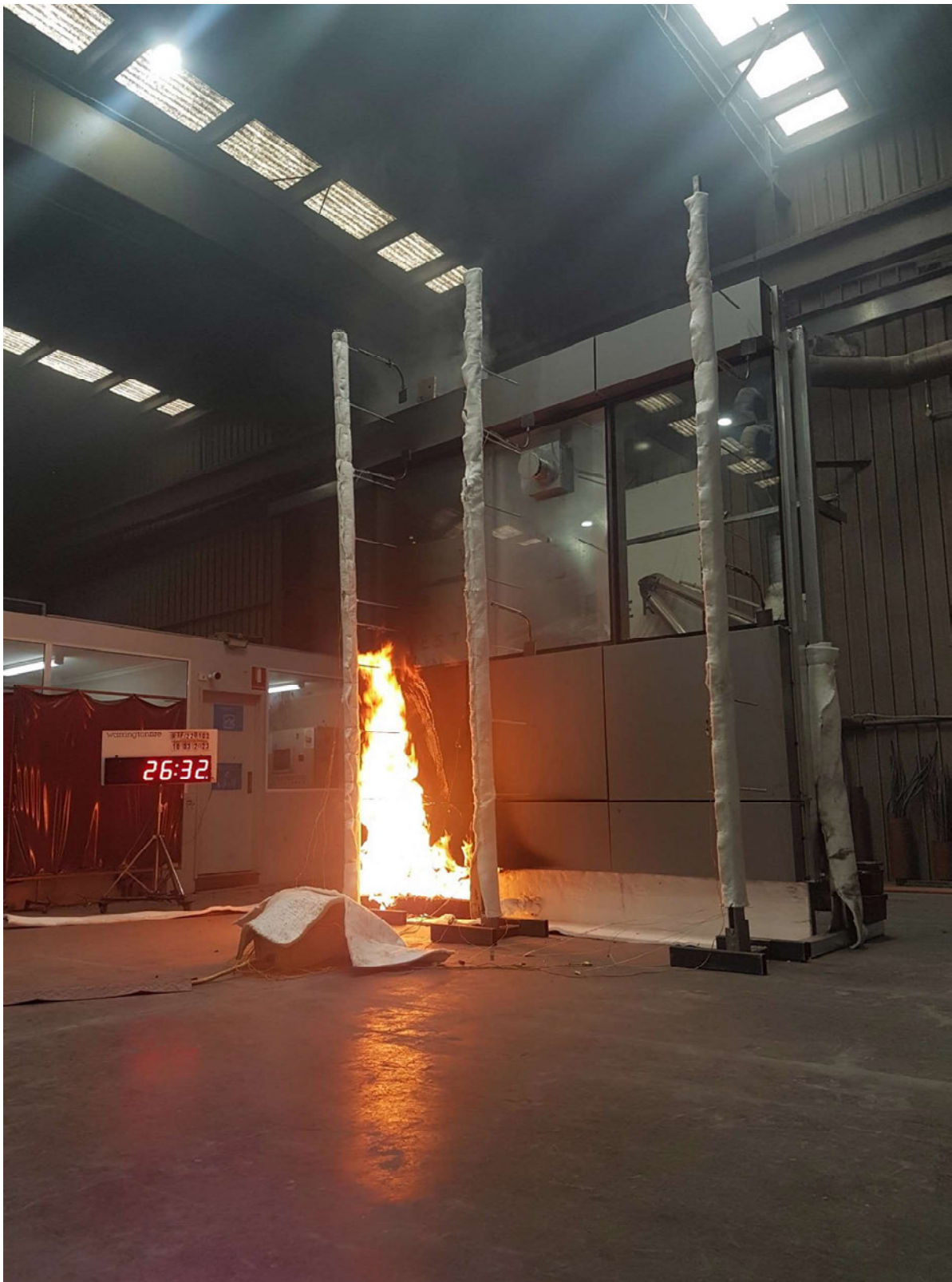
Figure 46 The specimen 26 minutes 32 seconds into the test (burner output at 300 kW)
