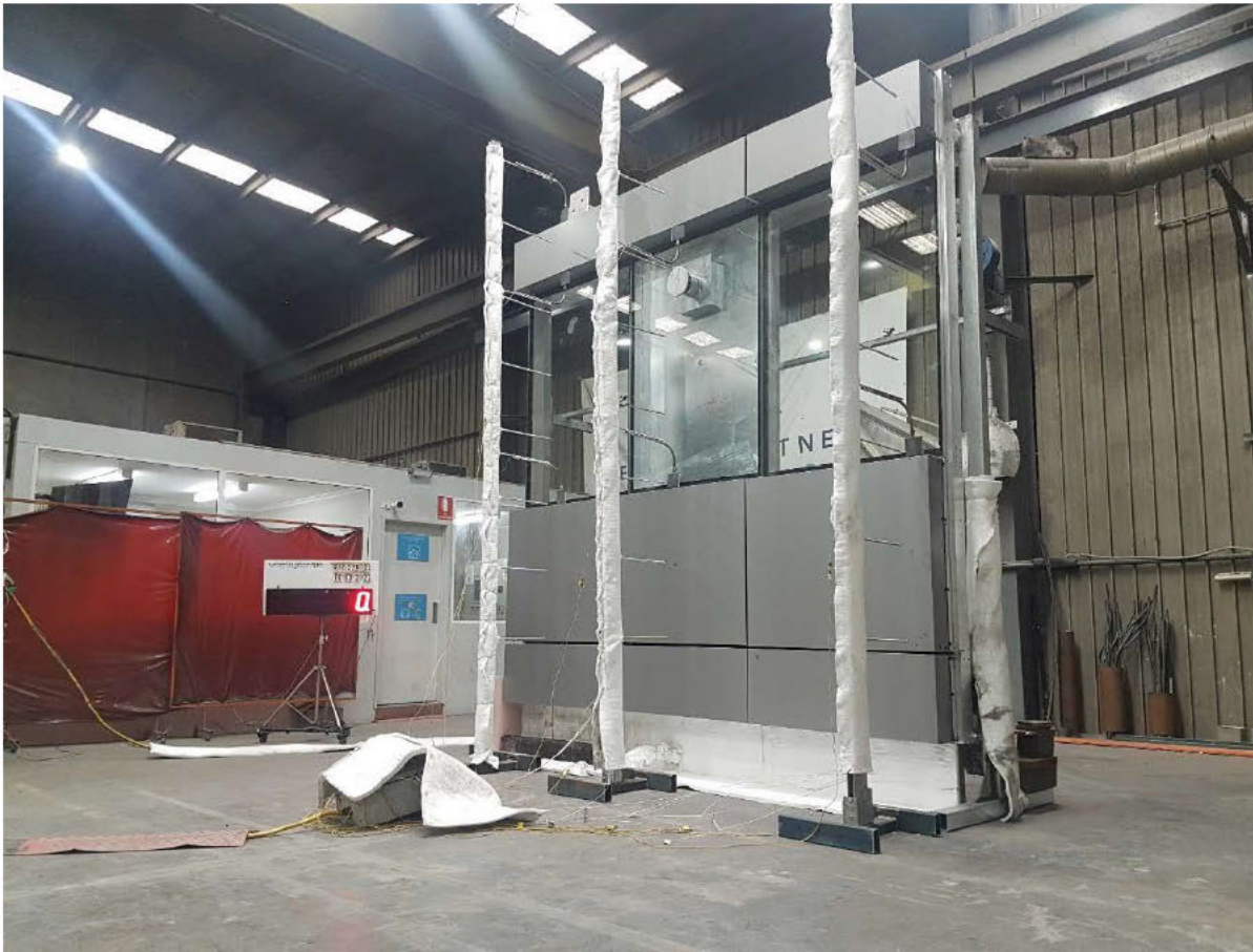
Figure 22 The specimen (angled - exposed side) before the reaction to fire test
