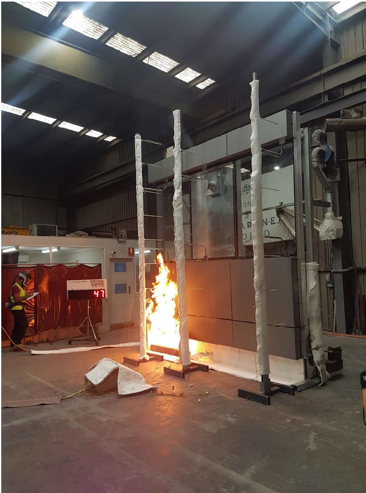
Figure 23 The specimen 47 seconds into the test (burner output at 300 kW)
