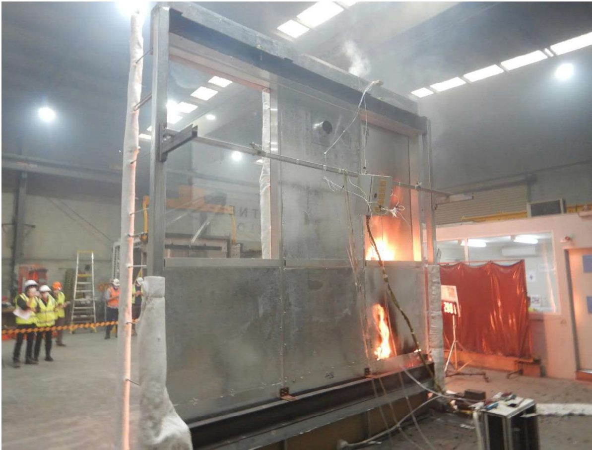
Figure 48 The specimen 28 minutes 1 second into the test (burner output at 300 kW) – unexposed side.
