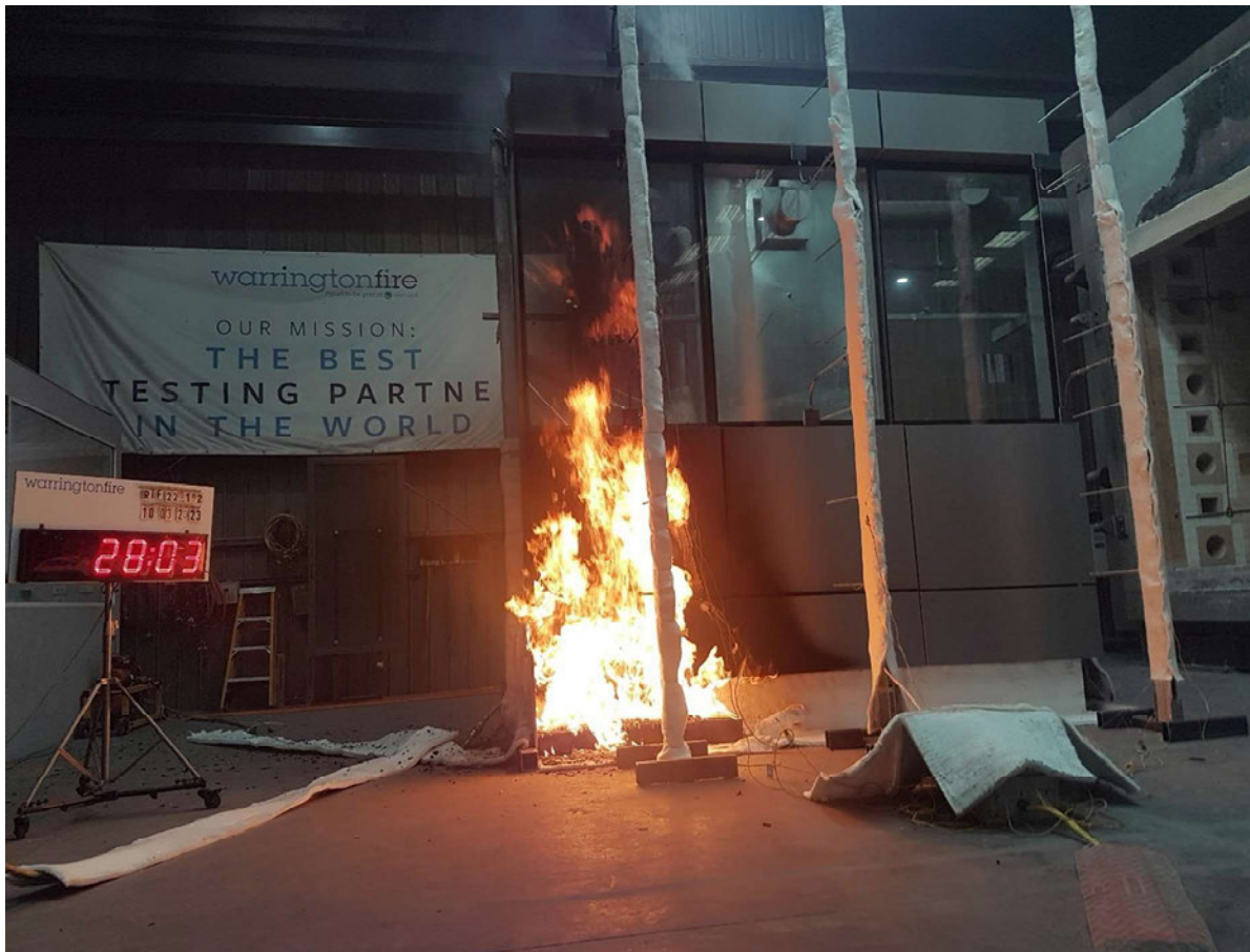
Figure 47 The specimen 28 minutes 3 seconds into the test (burner output at 300 kW)
