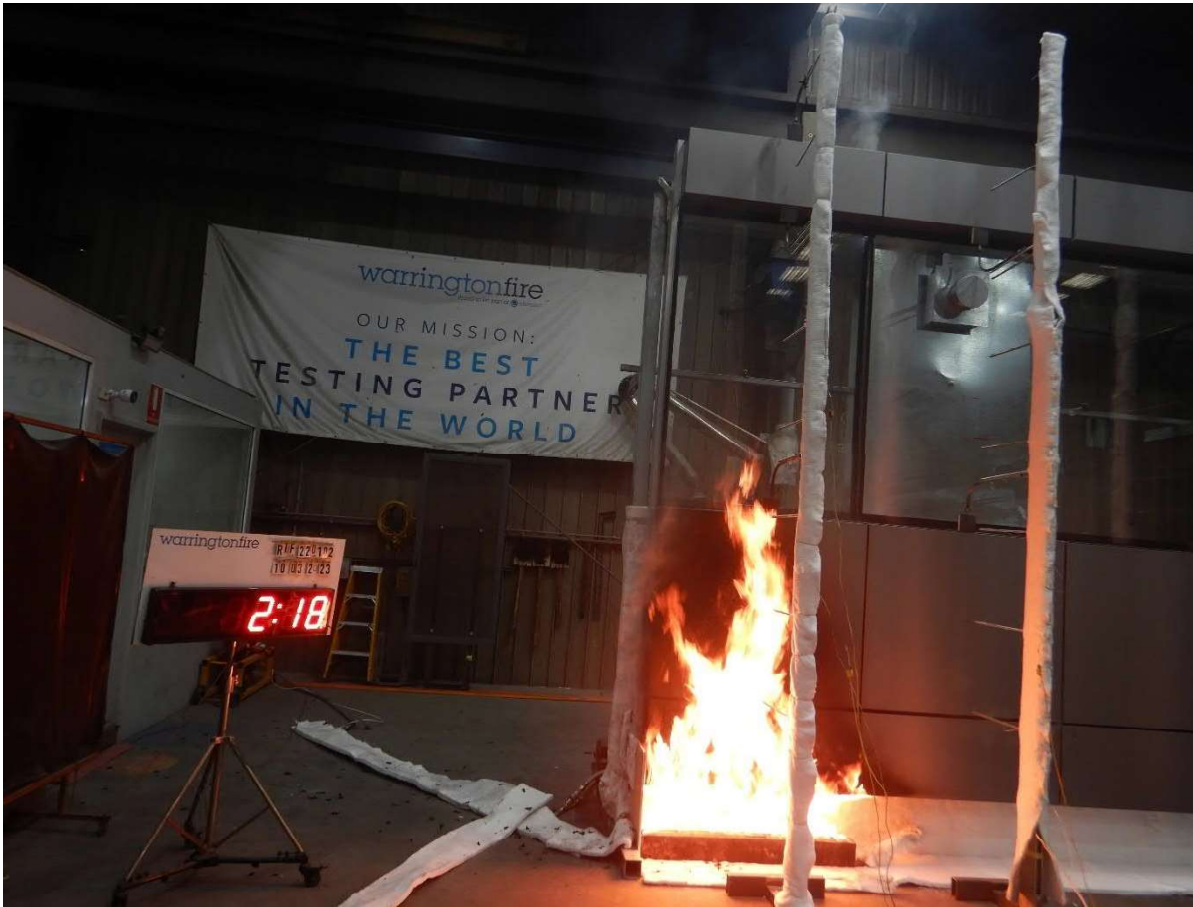
Figure 24 The specimen 2 minutes 18 seconds into the test (burner output at 300 kW)
