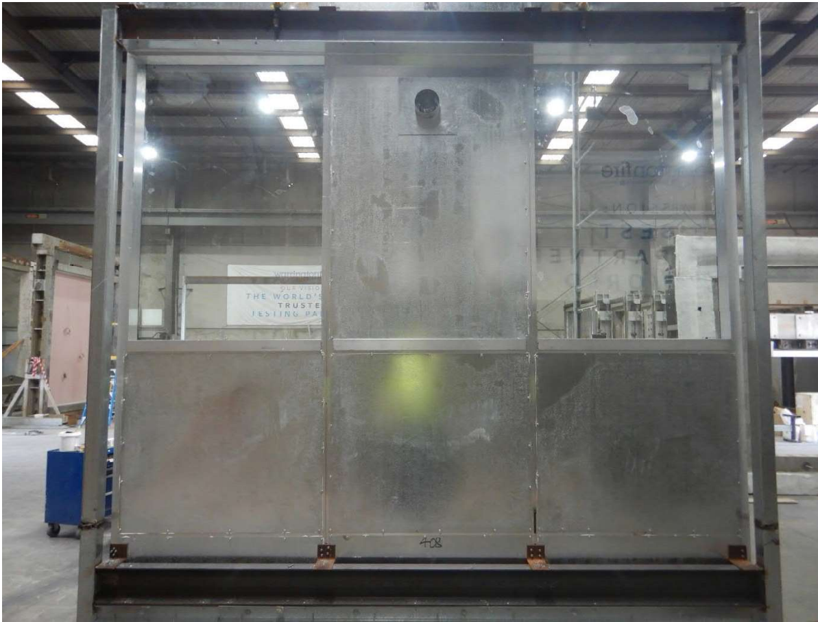
Figure 21 The specimen (unexposed side) before the reaction to fire test
