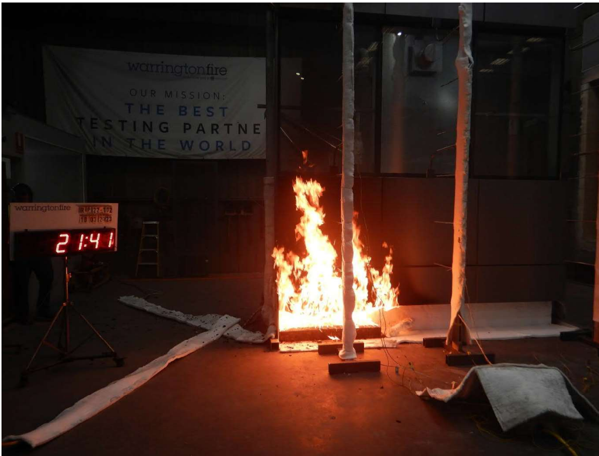
Figure 40 The specimen 21 minutes 41 seconds into the test (burner output at 300 kW)
