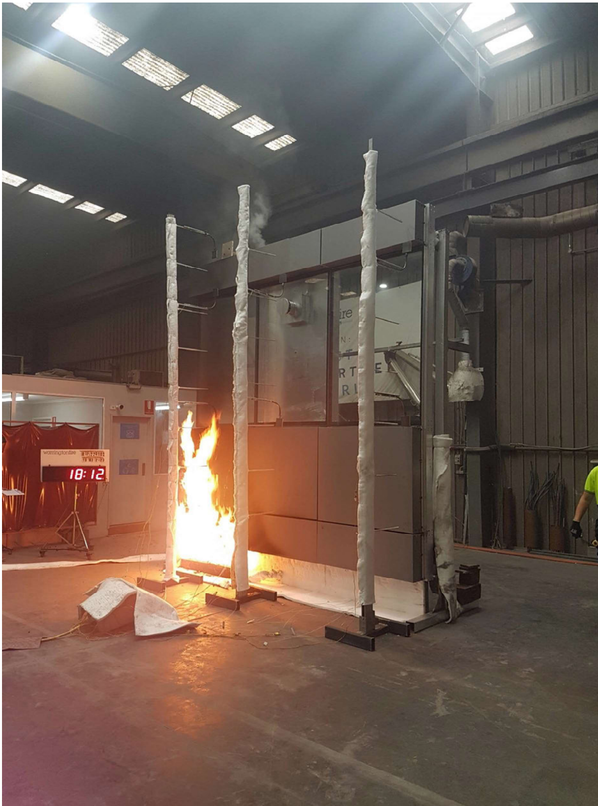
Figure 36 The specimen 18 minutes 12 seconds into the test (burner output at 300 kW)
