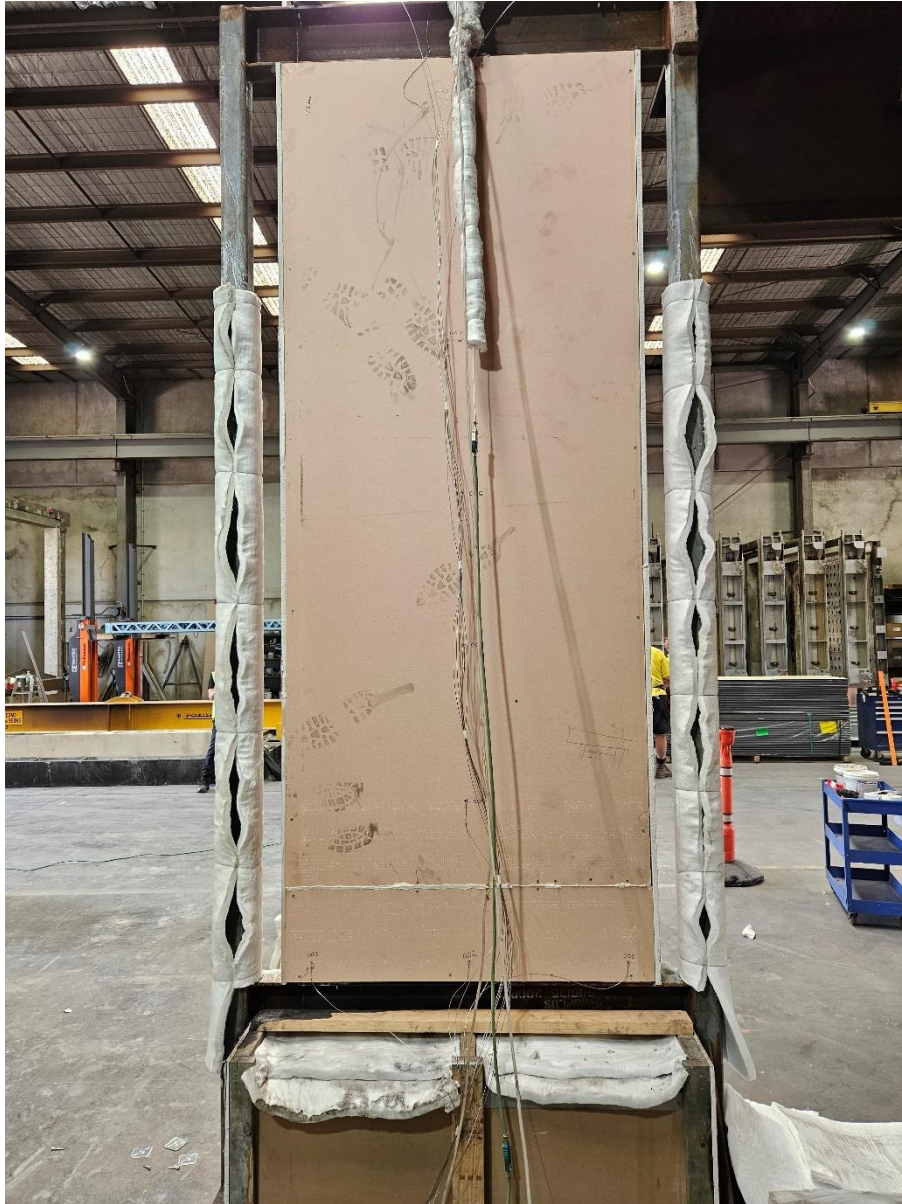
Figure 14 The specimen before the reaction to fire test – unexposed side
