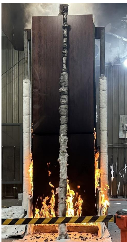
Figure 20 The specimen 39 minutes 42 seconds into the test (24 minutes 42 seconds after burner output was changed to 300 kW)
