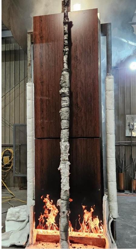
Figure 15 The specimen 12 minutes 56 seconds into the test (burner output at 100 kW)
