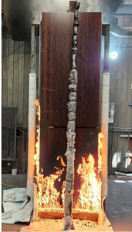
Figure 17 The specimen 15 minutes 30 seconds into the test (30 seconds after burner output was changed to 300 kW)
