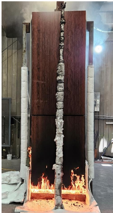
Figure 16 The specimen 14 minutes 59 seconds into the test (burner output at 100 kW)
