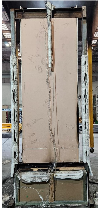
Figure 24 The specimen after the test – unexposed side.
