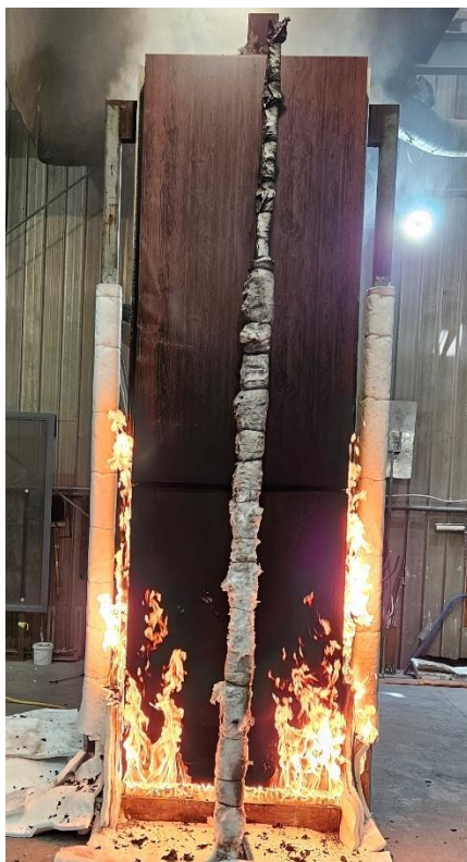
Figure 19 The specimen 33 minutes into the test (8 minutes after burner output was changed to 300 kW)
