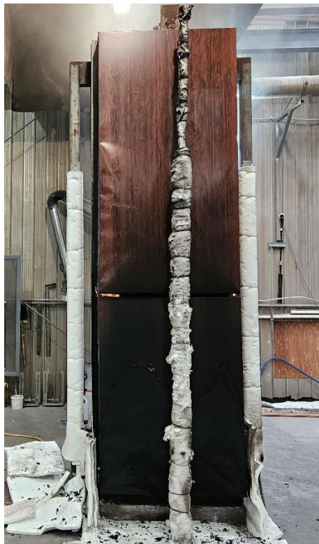
Figure 22 The specimen 50 minutes 3 seconds into the test (10 minutes 3 seconds after burner was switched off)
