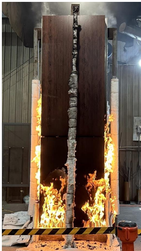
Figure 18 The specimen 20 minutes into the test (5 minutes after burner output was changed to 300 kW)
