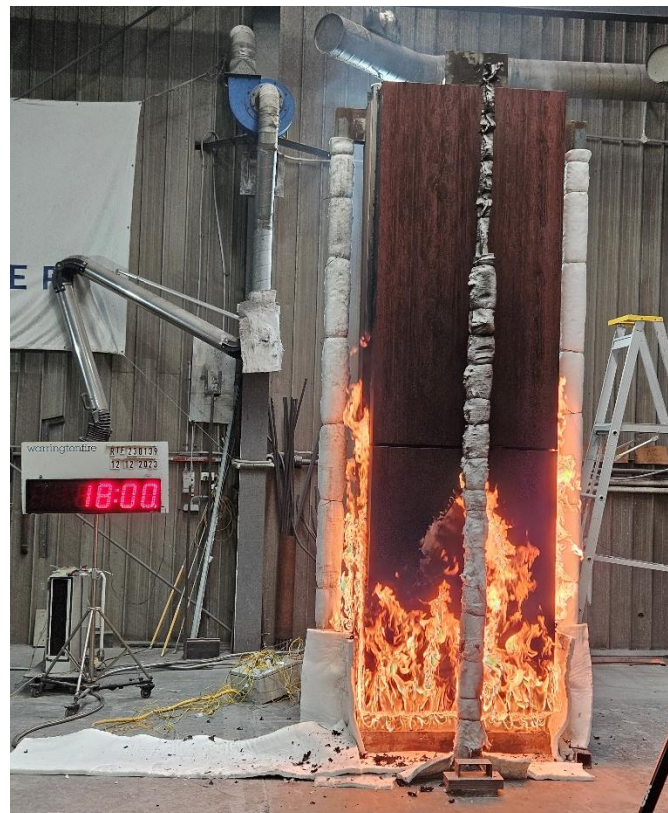
Figure 17 The specimen 18 minutes into the test (3 minutes after burner output was changed to 300 kW)
