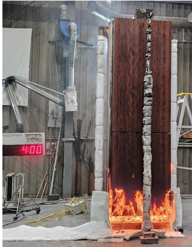
Figure 14 The specimen 4 minutes into the test (burner output at 100 kW)
