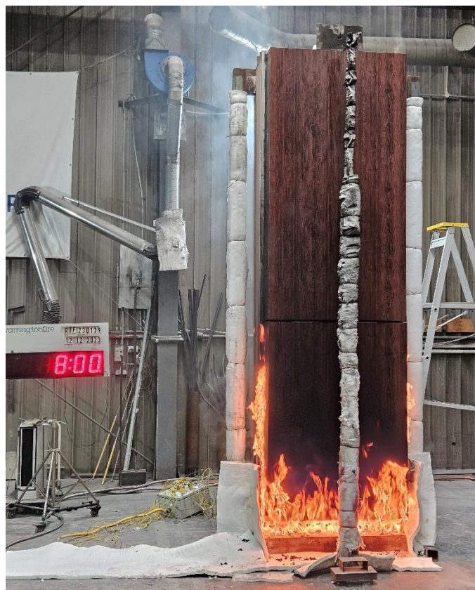
Figure 15 The specimen 8 minutes into the test (burner output at 100 kW)
