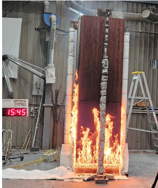
Figure 16 The specimen 15 minutes 45 seconds into the test (45 seconds after burner output was changed to 300 kW)
