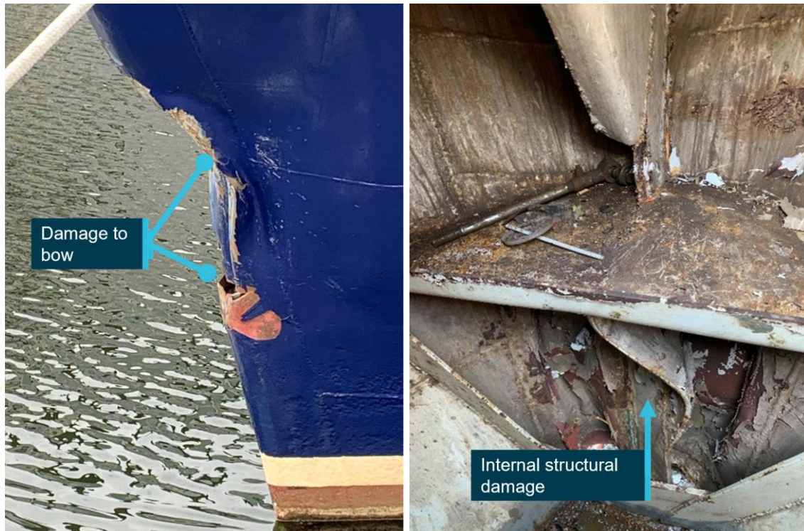
Figure 2: Impact damage to Lady Cutler's bow
