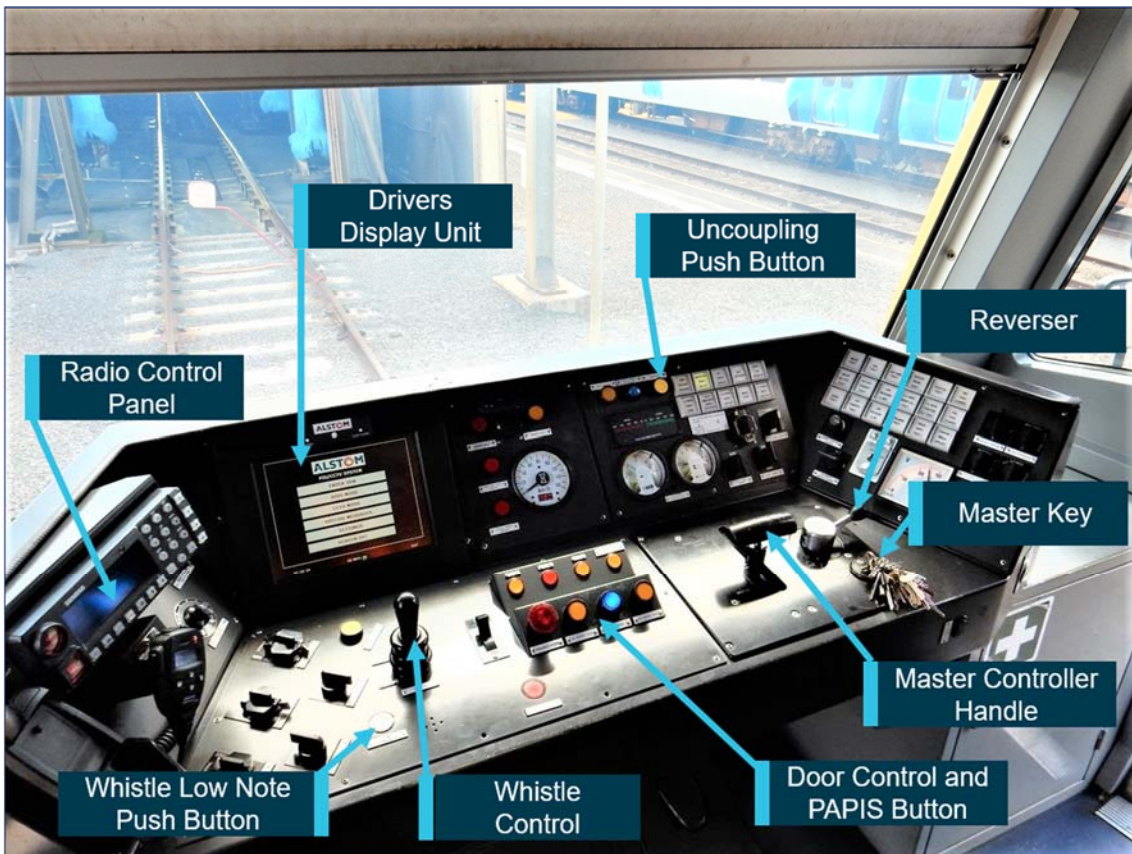
Figure 4: Master Controller Panel
