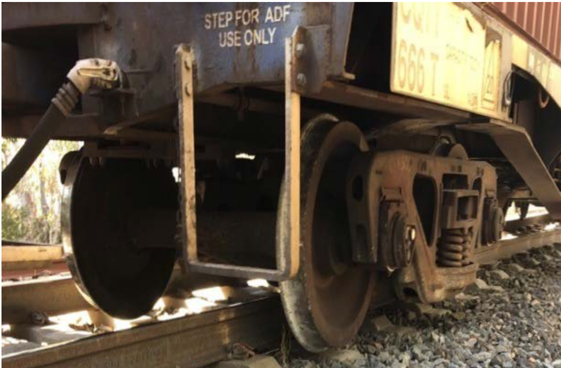
Figure 2: Derailed bogie of wagon CQTY 666T
