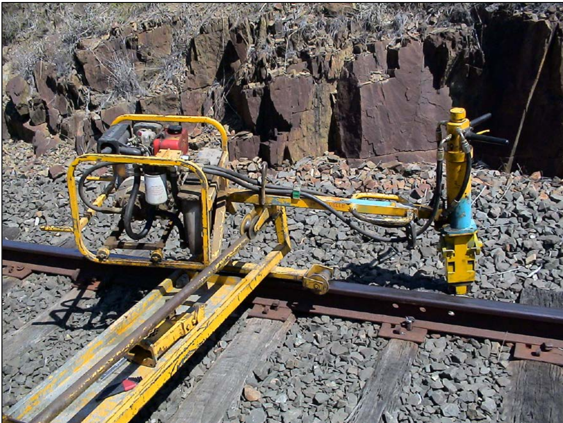
Figure 1: A dog spike puller similar to that used at Montgomery
