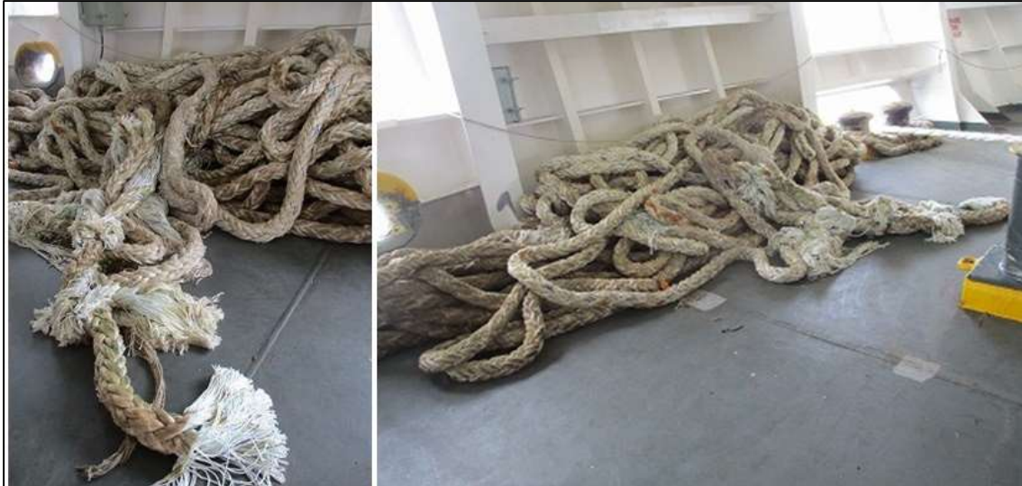
Figure 7: Photographs of damaged mooring lines.
