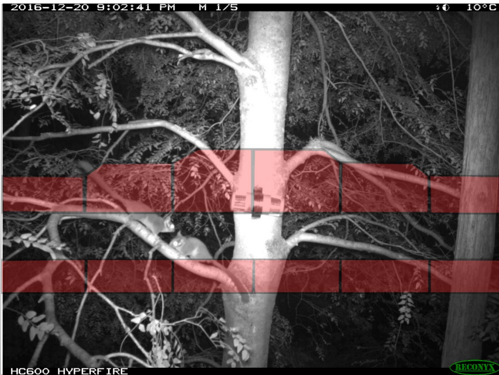
Images above: Examples of LBP camera alignment with bait stations and the location of the PIR sensor
