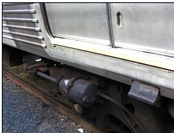
Figure 3 – Comeng motor car, showing door used by victim and proximate car brake cylinder (see photo below).
