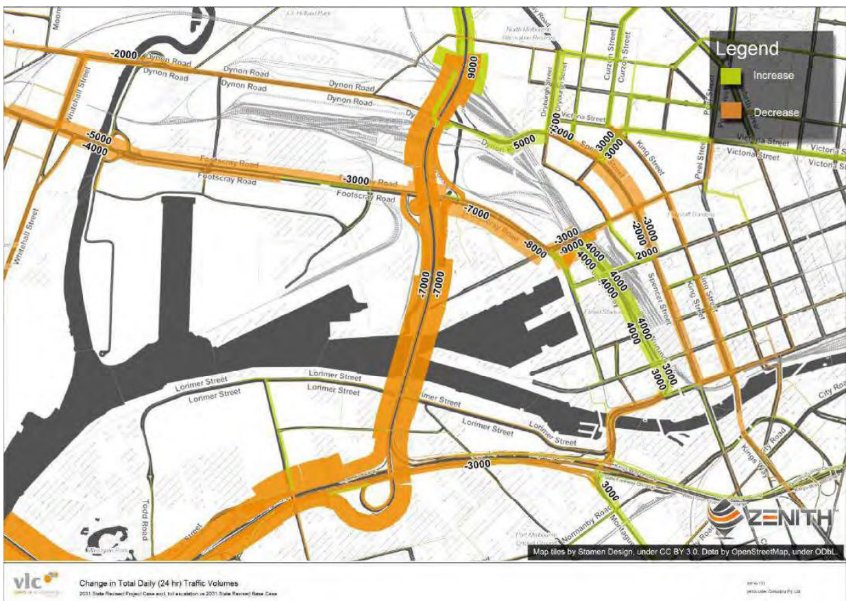
Figure 47 - Western Distributor impact on city routes over 24 hours (2031 project case vs 2031 base case)
